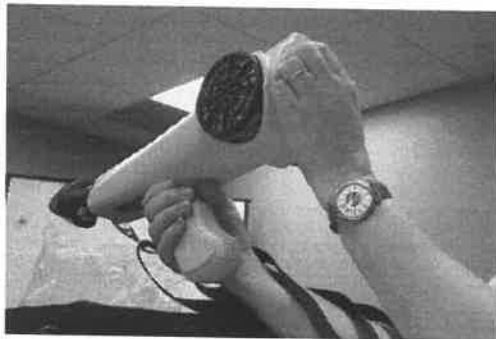
A Nasal Ranger, a device that measures the odors in the air. It is in use in Colorado, the first state to legalize recreational marijuana. Dave Kolpack/Associated Press
