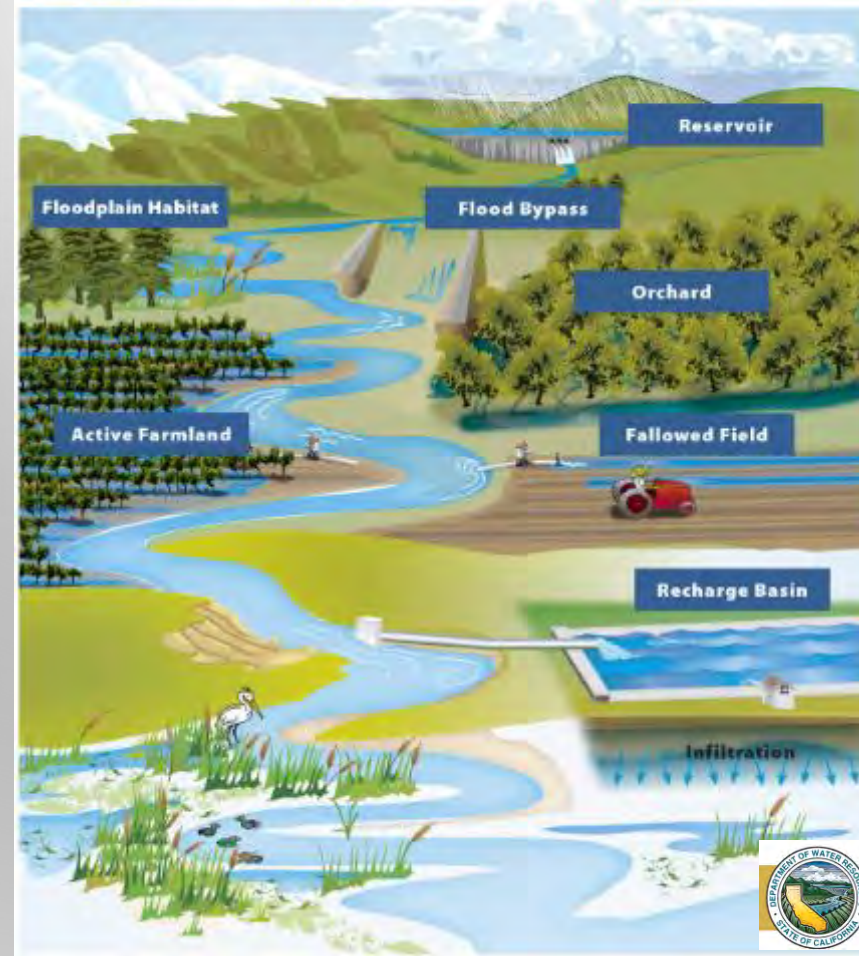
Example areas of managed aquifer recharge (MAR)
