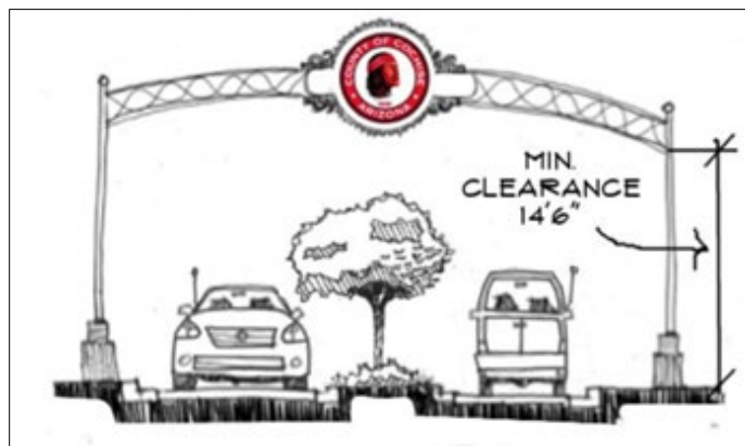
Figure 10. A minimum clearance of 14.5' is required under all arches, signs and underpasses.
