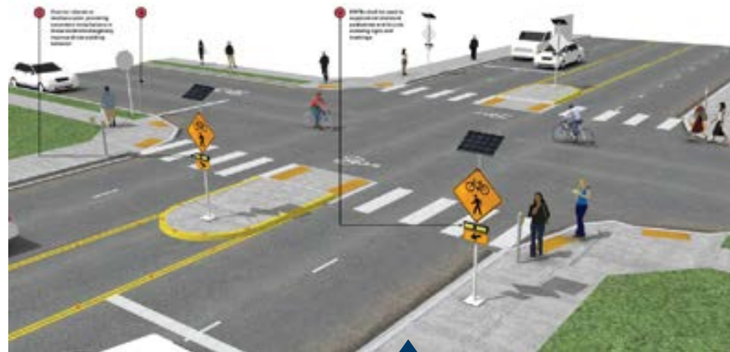
Graphic illustrating design of RRFB intersections Source: NACTO, "Urban Bikeway Design Guide" National Association of City Transportation Officials
