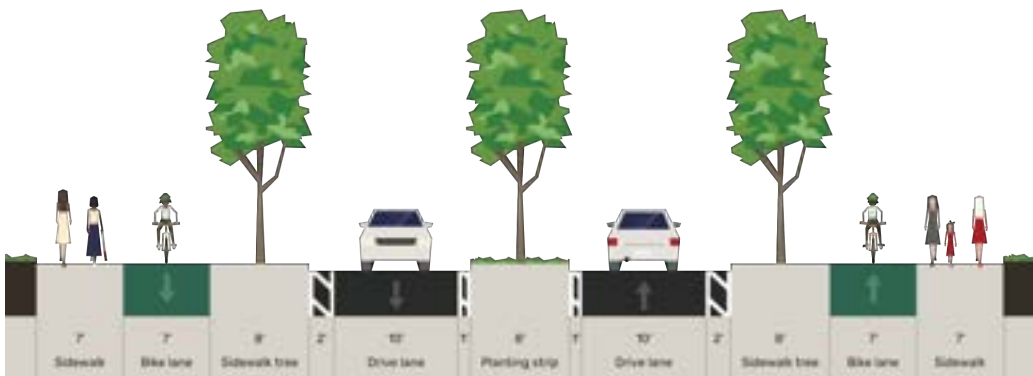
Full Build Cross Section | 78' Right of Way
