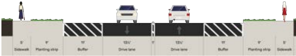
Existing Cross Section | 78' Right of Way
