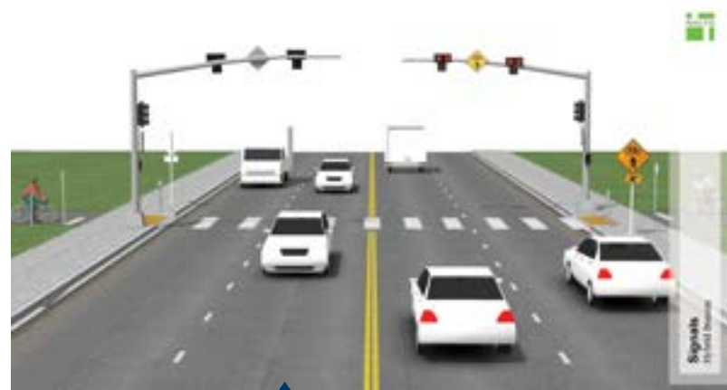
Graphic illustrating design of PHB intersections Source: NACTO, "Urban Bikeway Design Guide" National Association of City Transportation Officials
