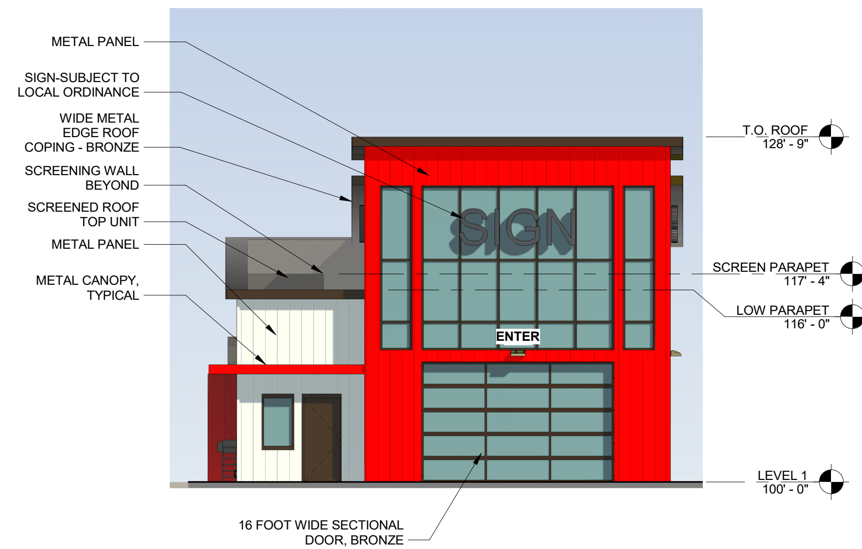
2 WEST ELEVATION 1/8" = 1'-0"
