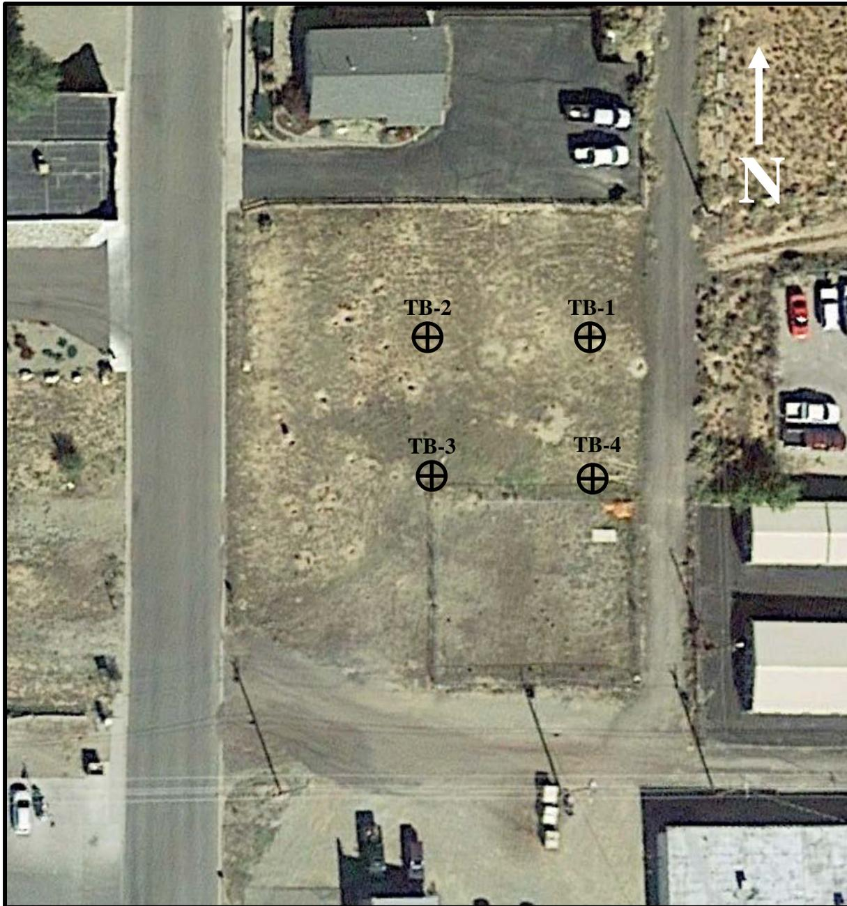
The schematic presented above was prepared using notes and field measurements obtained during our field exploration and is intended to show the approximate test boring locations for reference purposes only.
