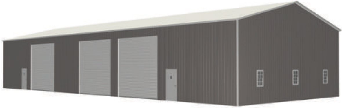
Computer-generated drawing of 110' x 40' x 16' pre-fab steel building
