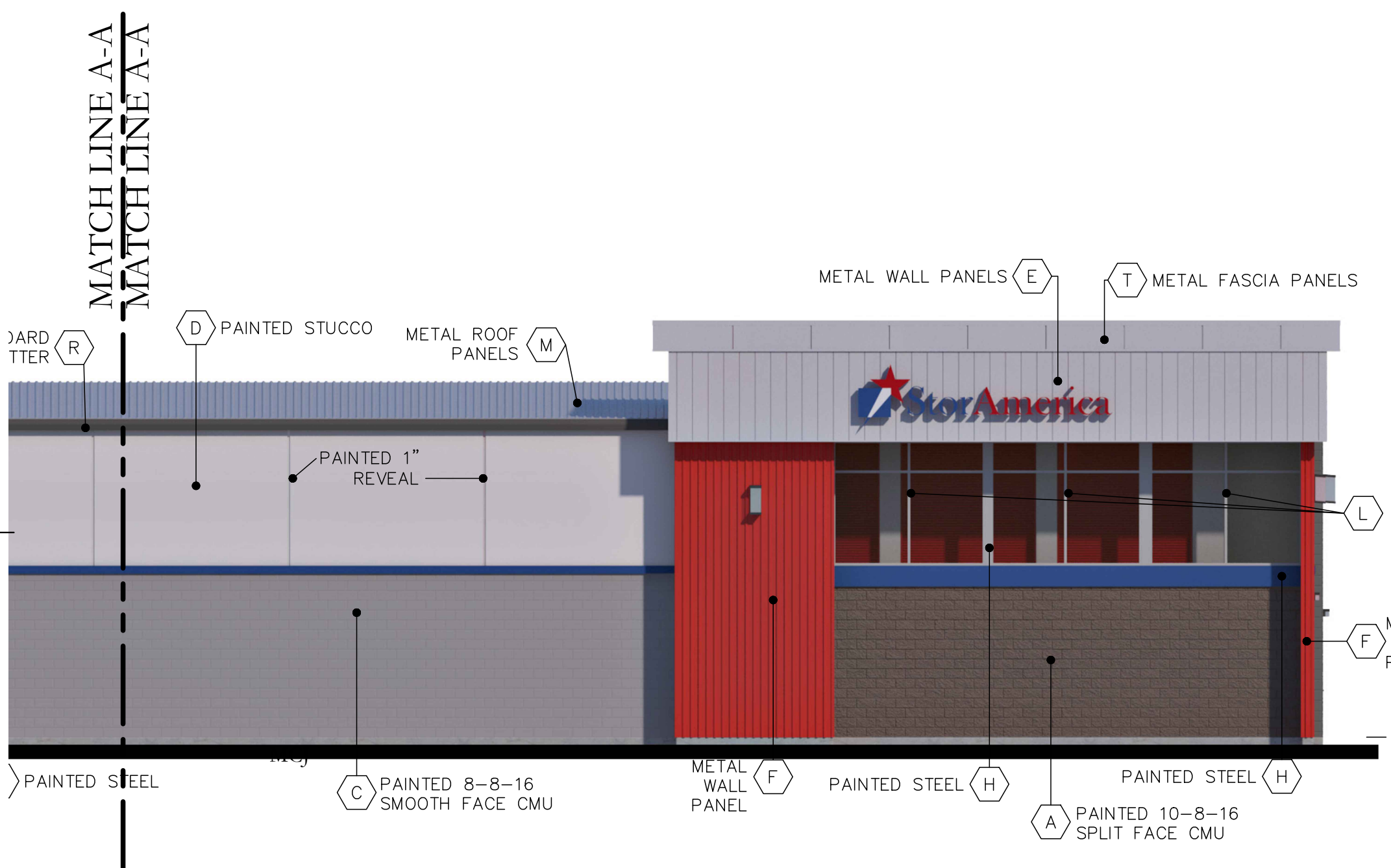
BUILDING B- NORTH ELEVATION- cont. SCALE: 1/8" = 1'-0"
