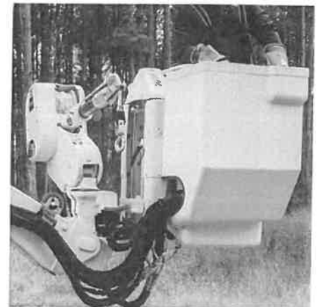
24" PLATFORM ELEVATOR OPTIMIZES OPERATOR REACH WITHIN WORK ZONE
