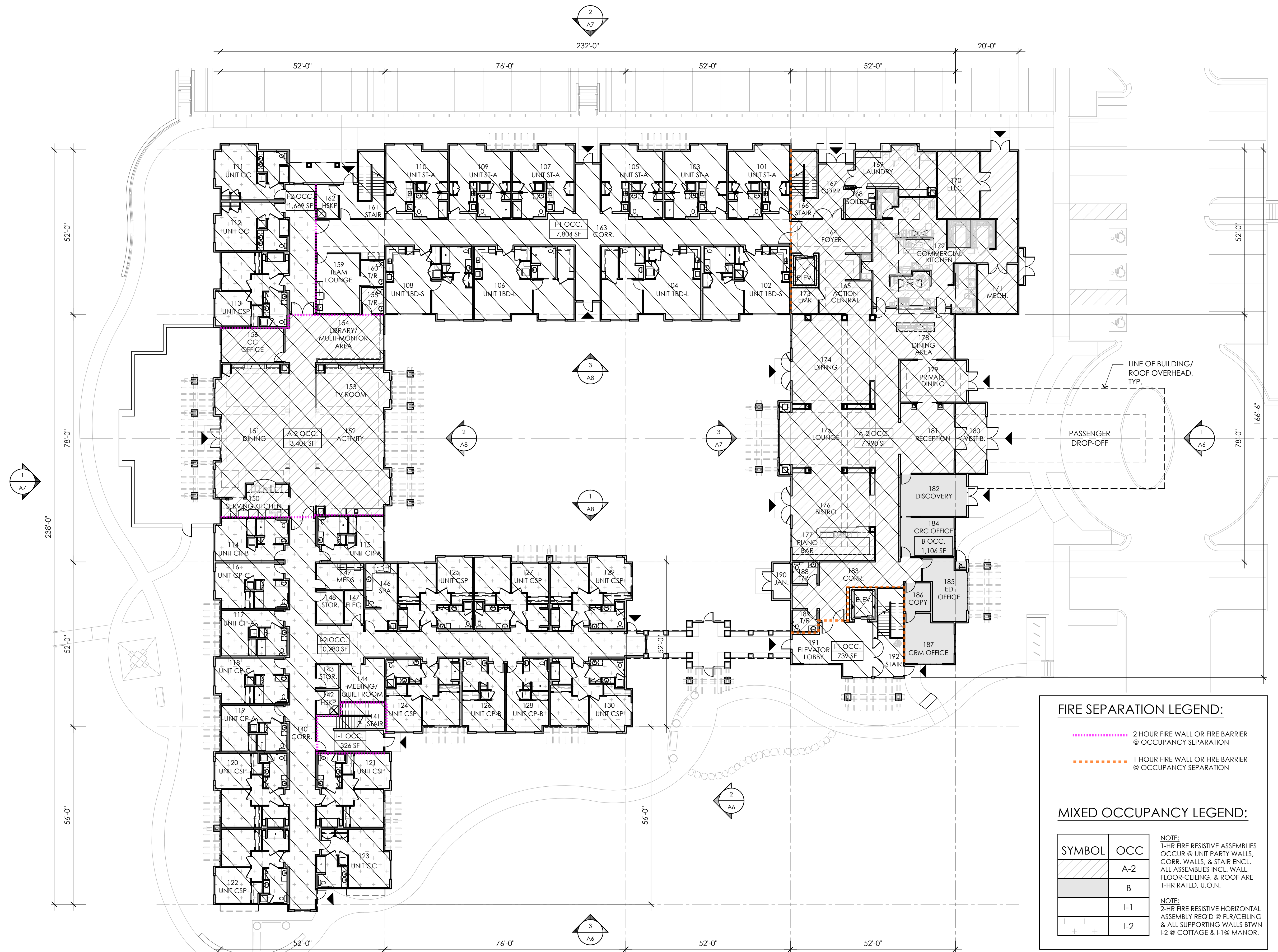
1 FIRST FLOOR PLAN FINISH FLOOR ELEV. = +7075' DATUM ELEV. = +0'-0" 1/16" = 1'-0" NORTH
