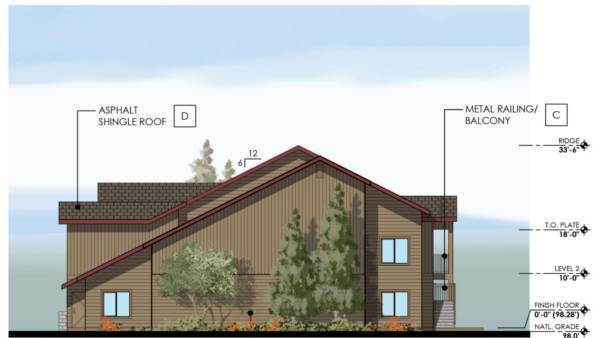
BUILDING TYPE 1 EAST ELEVATION
