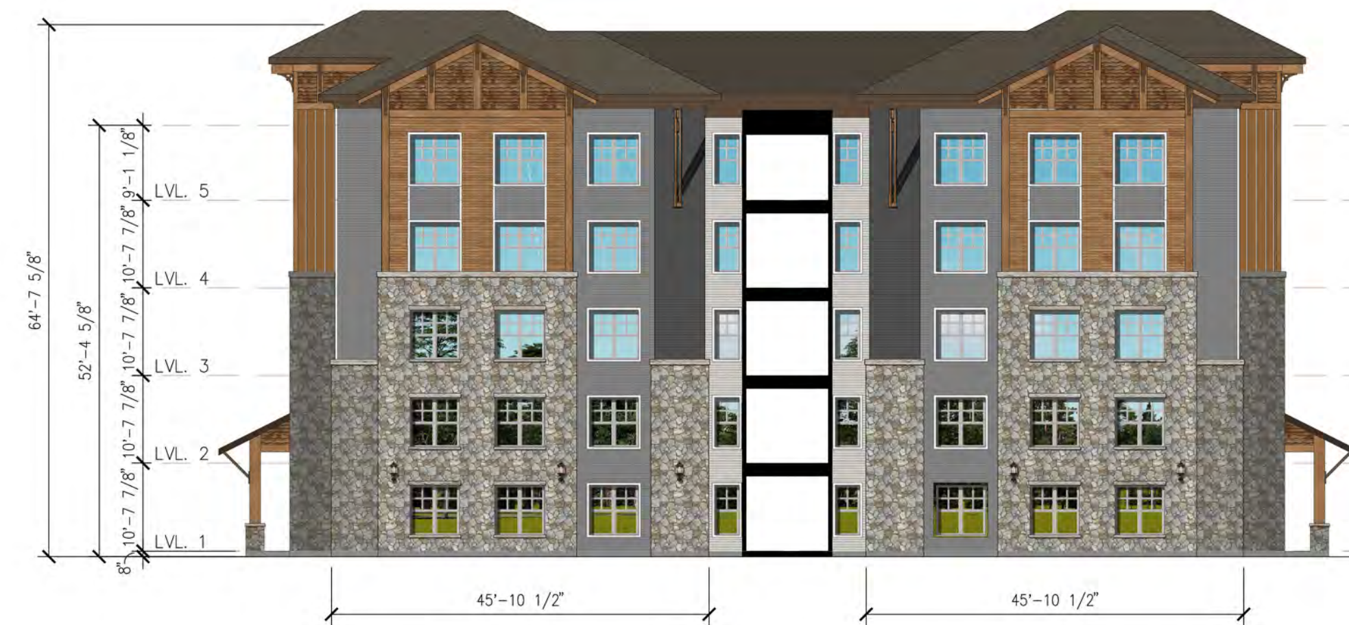
2 COURTYARD 1 - EAST ELEVATION 1/16"=1'-0" BUILDING 2
