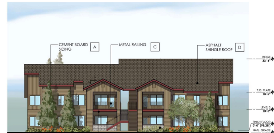
BUILDING TYPE 1 EAST ELEVATION
