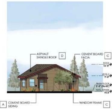
BUILDING TYPE 3 SOUTH ELEVATION 3/32" = 1'-0"
