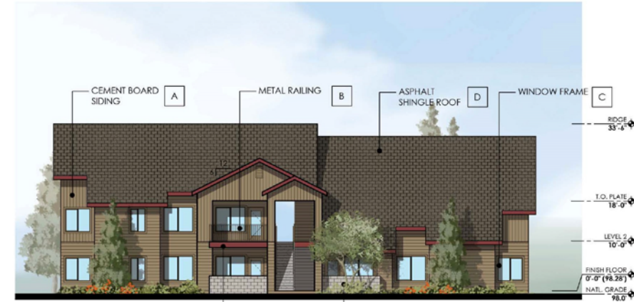
BUILDING TYPE 1 WEST ELEVATION - IZABEL STREET
