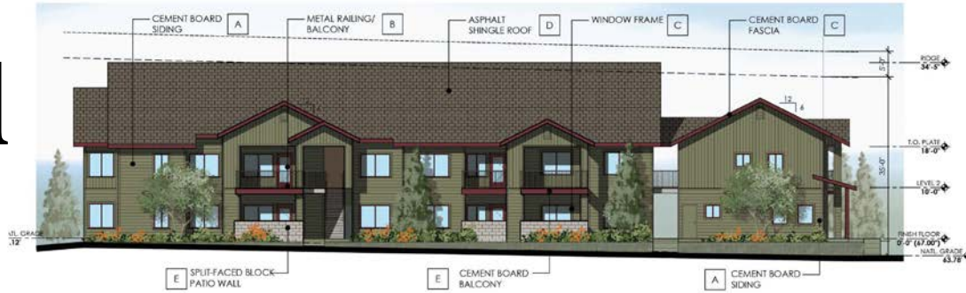
WEST ELEVATION - N. WEST STREET
