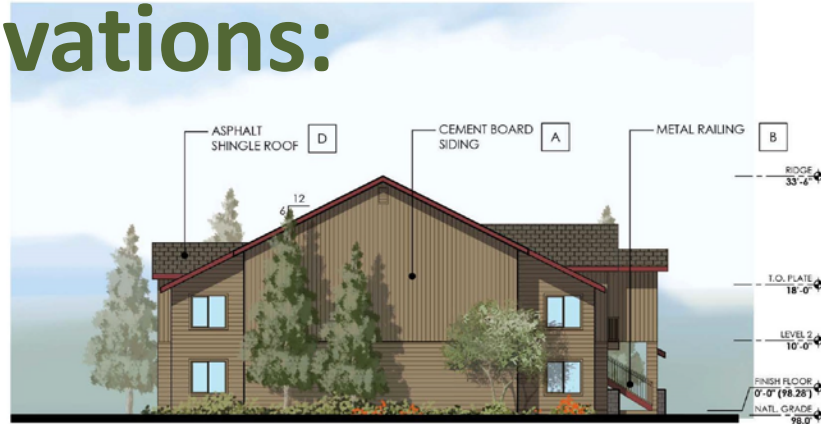
BUILDING TYPE 1 NORTH ELEVATION - COLANTHE AVENUE
