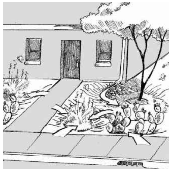
EXAMPLE OF HARVESTING RAINWATER BY DIRECTING RUNOFF TO LANDSCAPED AREAS. (GRAPHIC COURTESY OF BRAD LANCASTER AND WWW.RAINWATERHARVESTING.COM)
