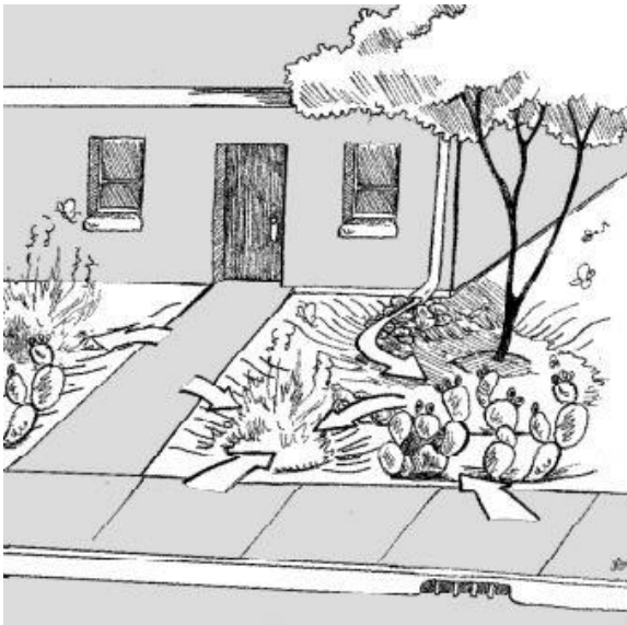
Example of harvesting rainwater by directing runoff to landscaped areas.
