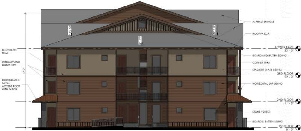
E1 SOUTH ELEVATION SCALE: 1/8" = 1'-0"
