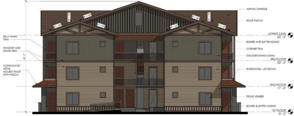
E1 SOUTH ELEVATION SCALE: 1/8" = 1'-0"
