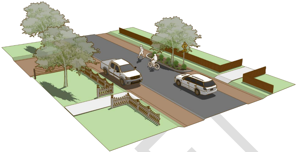
Figure 45: Yield Street Illustration from the Small Town and Rural Multimodal Networks Guide. (FHWA 2016)
