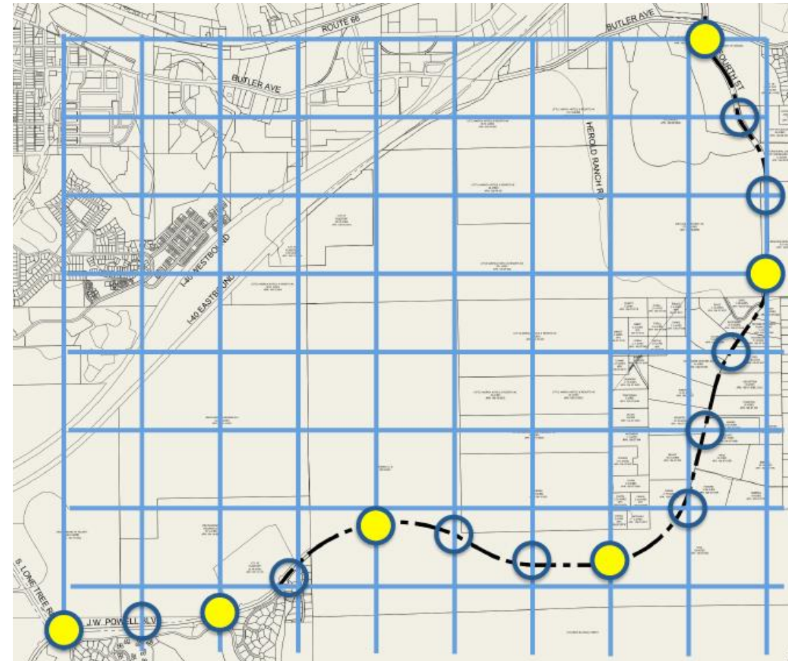
Depiction of a 1/4 mile transportation grid. Yellow dots are major intersections or activity nodes.
