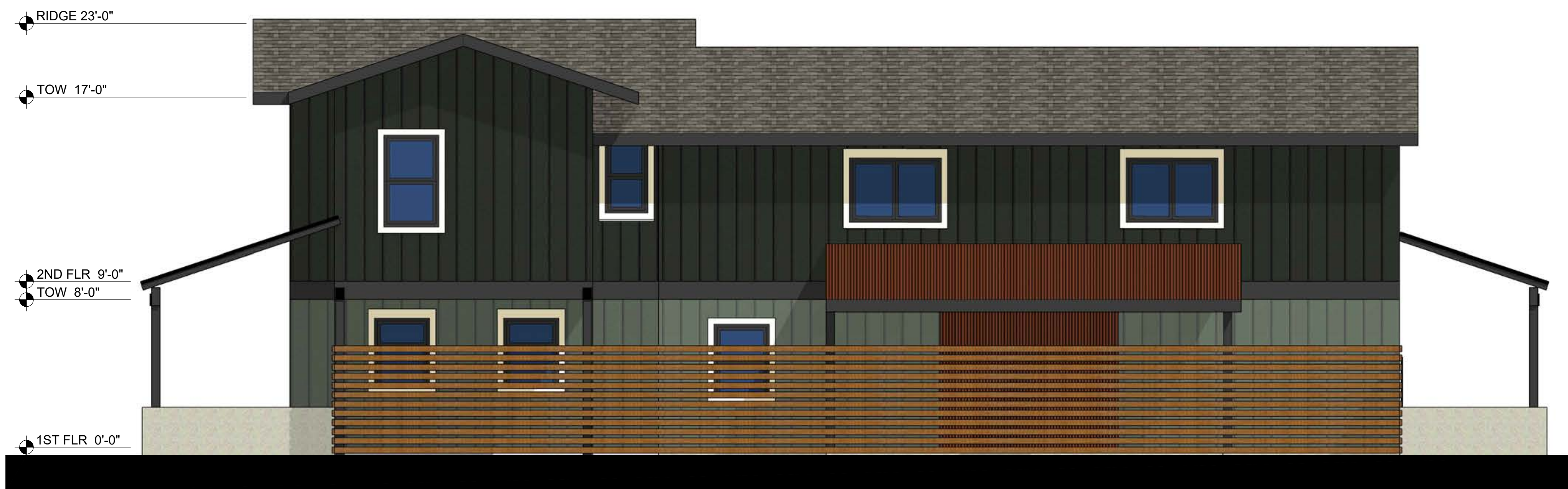
PROPOSED SIDE (WEST) ELEVATION SCALE: 1/4" = 1'-0"
