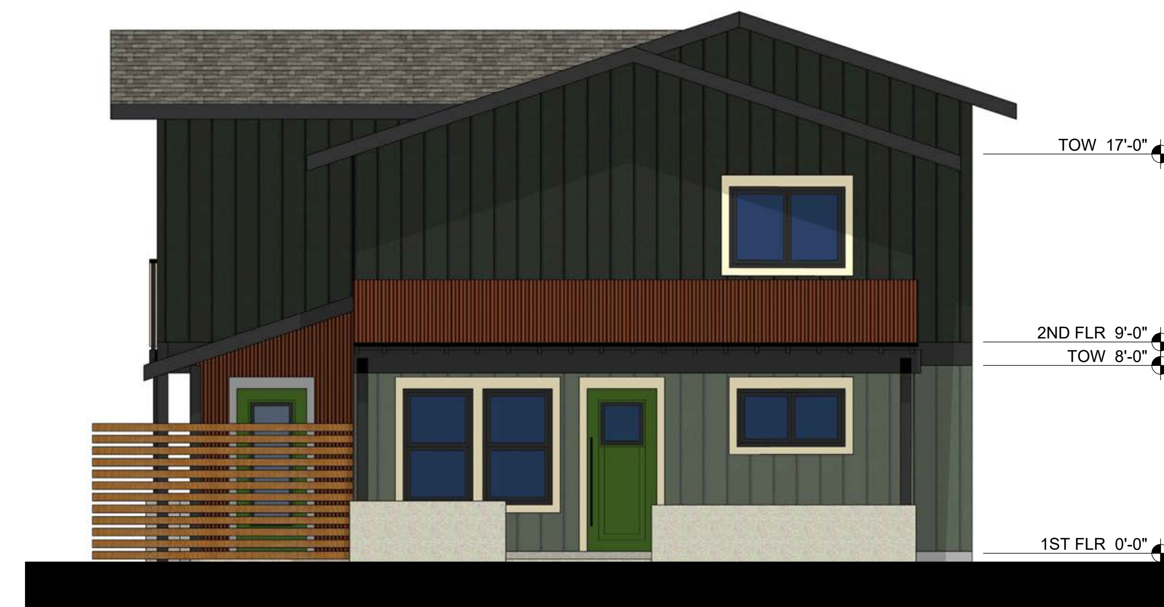
PROPOSED FRONT (SOUTH) ELEVATION SCALE: 1/4" = 1'-0"
