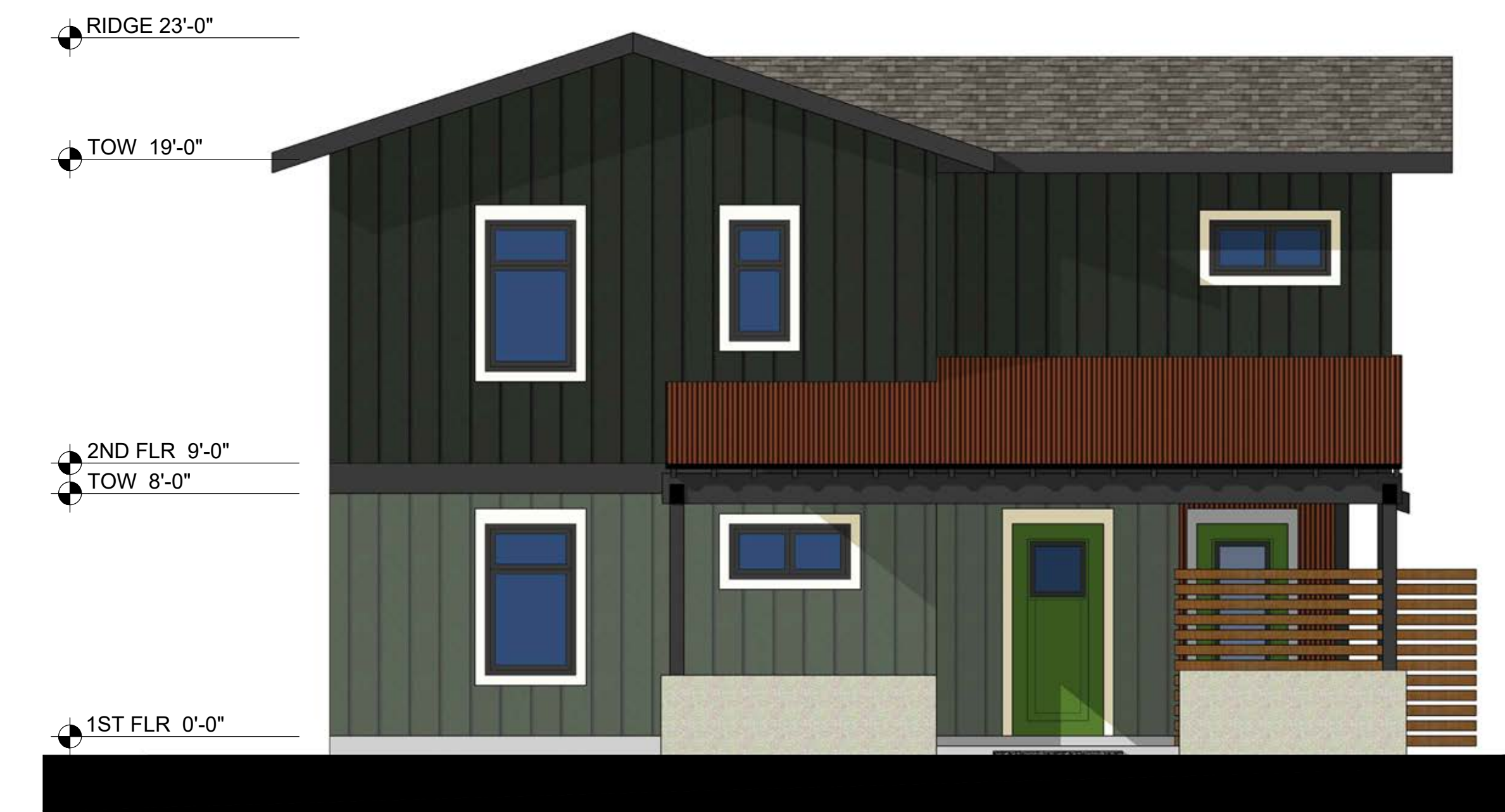
PROPOSED REAR (NORTH) ELEVATION SCALE: 1/4" = 1'-0"
