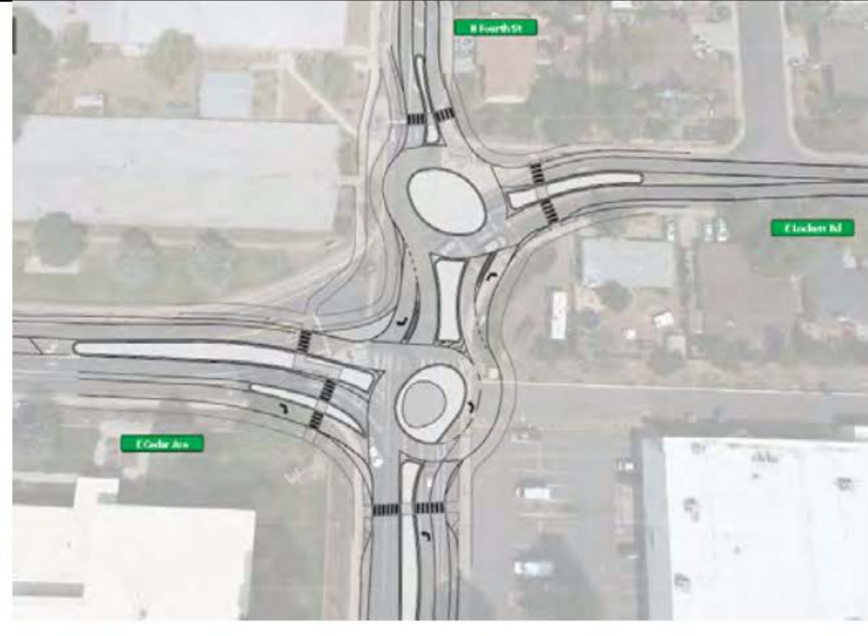
Alt C-4: Double Roundabout – No Residential Impacts South 100' x 90' ICD, North 100' x 80' ICD
