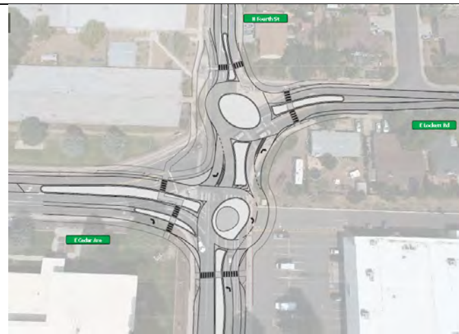
Alt C-4: Double Roundabout – No Residential Impacts South 100' x 90' ICD, North 100' x 80' ICD
