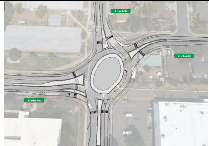
Alt C-4: Double Roundabout – No Residential Impacts South 100' x 90' ICD, North 100' x 80' ICD
