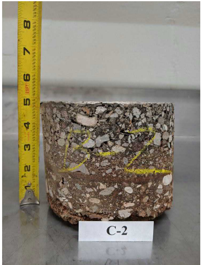
Photo No. 2: Asphalt core from boring location B-2
