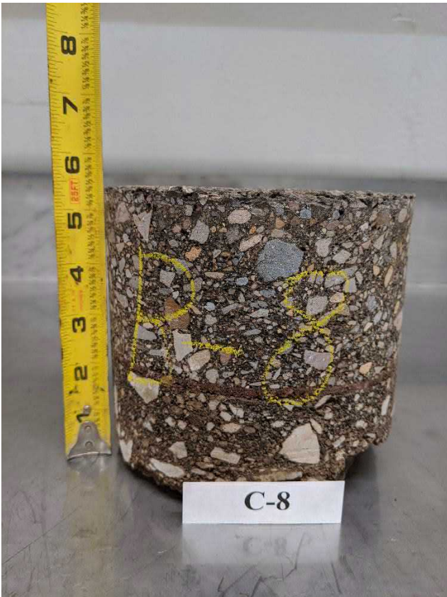
Photo No. 3: Asphalt core from boring location B-8
