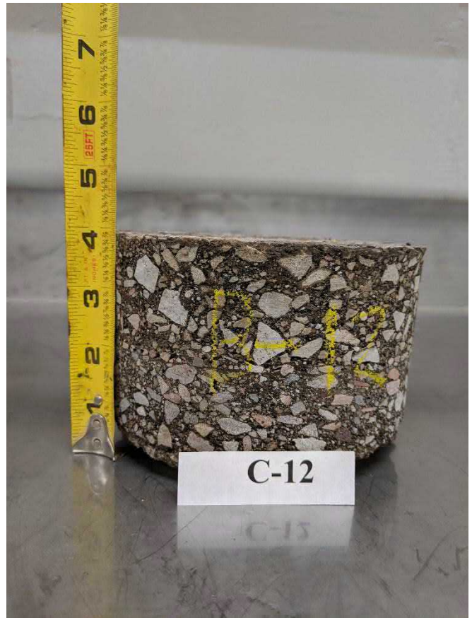
Photo No. 2: Asphalt core from boring location B-12
