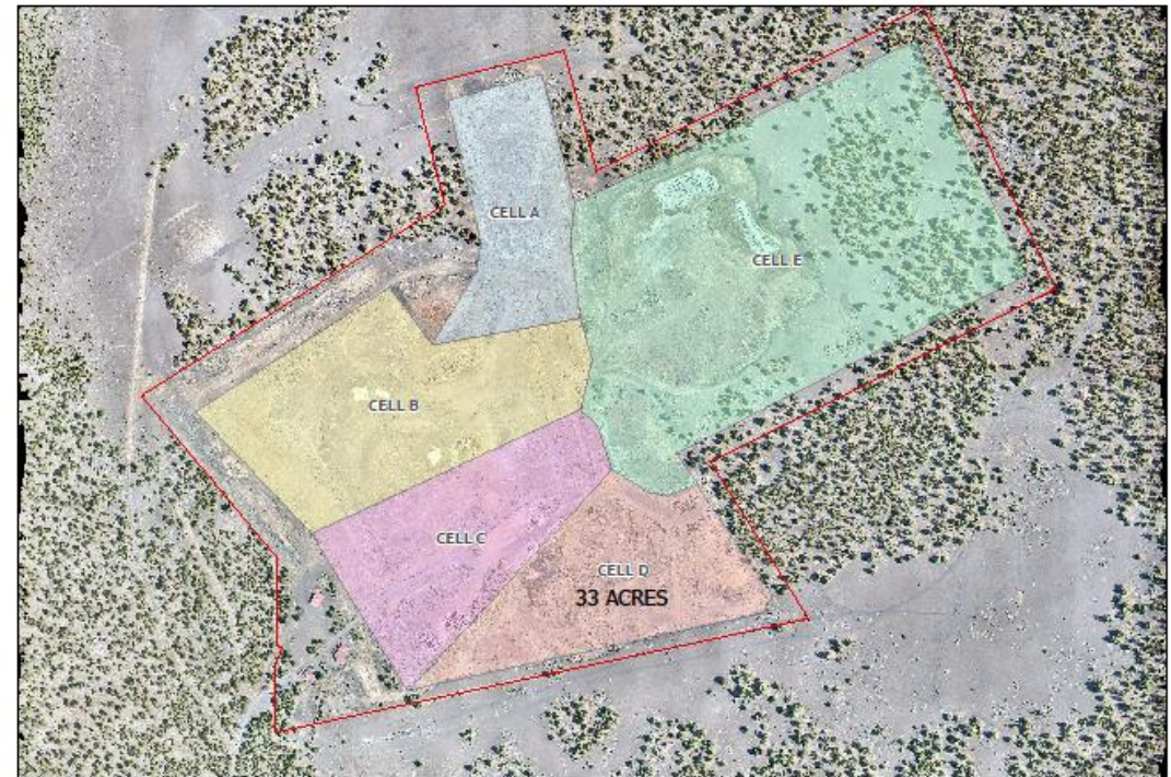
CINDER LAKE LANDFILL-SITE PLAN CELL/SEQUENCE D EXCAVATION
