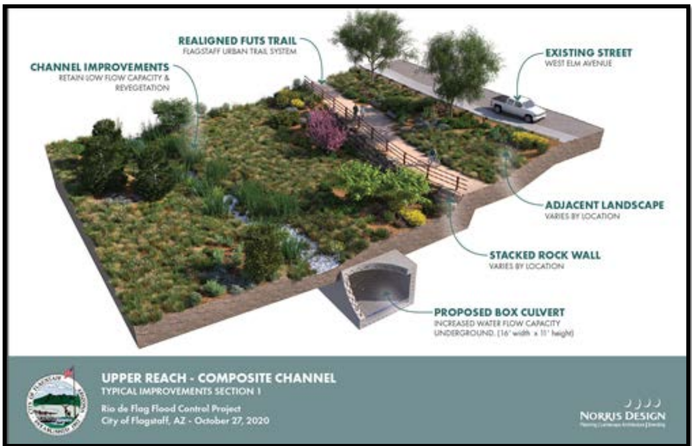
Upper Reach Composite Channel Concept
