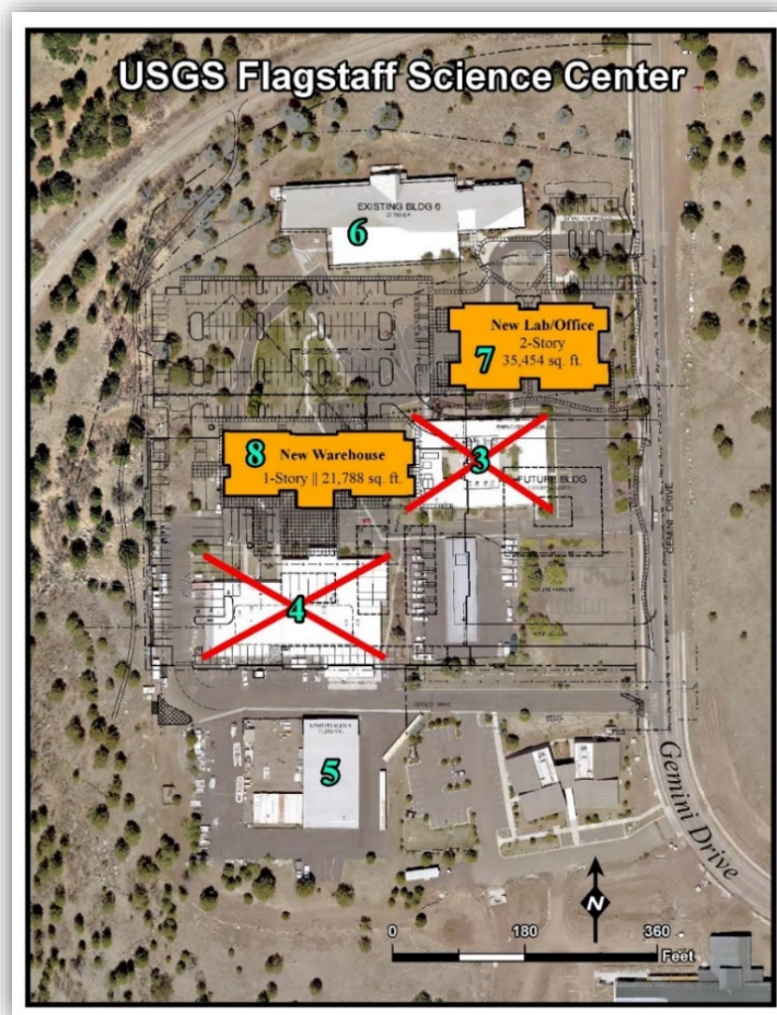
USGS Flagstaff Science Center Campus. Buildings to be constructed are shown in orange. Buildings 3 and 4 (shown with red X) will be demolished.
