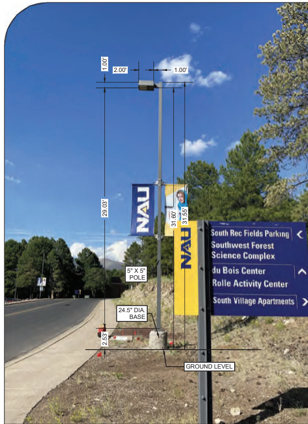
STREET LIGHT POLE DETAIL N.T.S.
