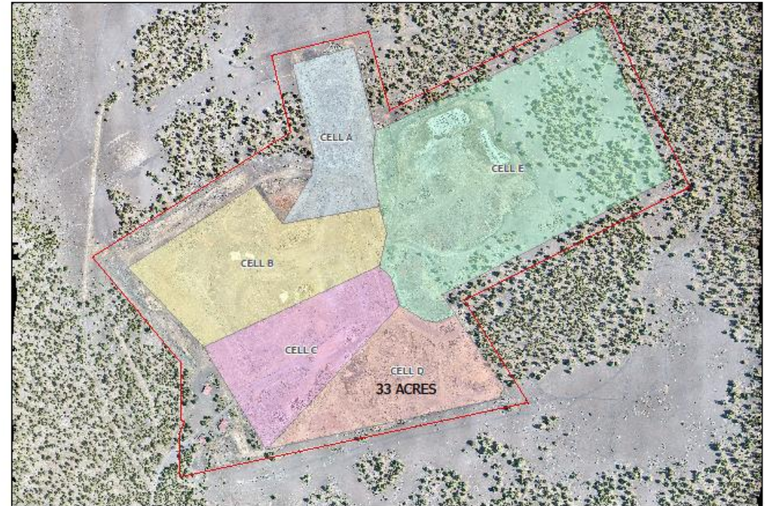
CINDER LAKE LANDFILL-SITE PLAN CELL/SEQUENCE D EXCAVATION
