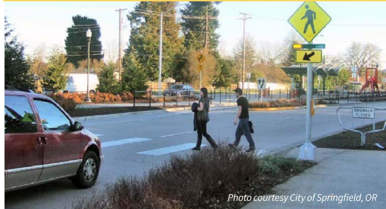
Fig. 2 Rectangular Rapid Flashing Beacon (RRFB) at Crossing Martin Luther King Roundabout, Springfield, OR
