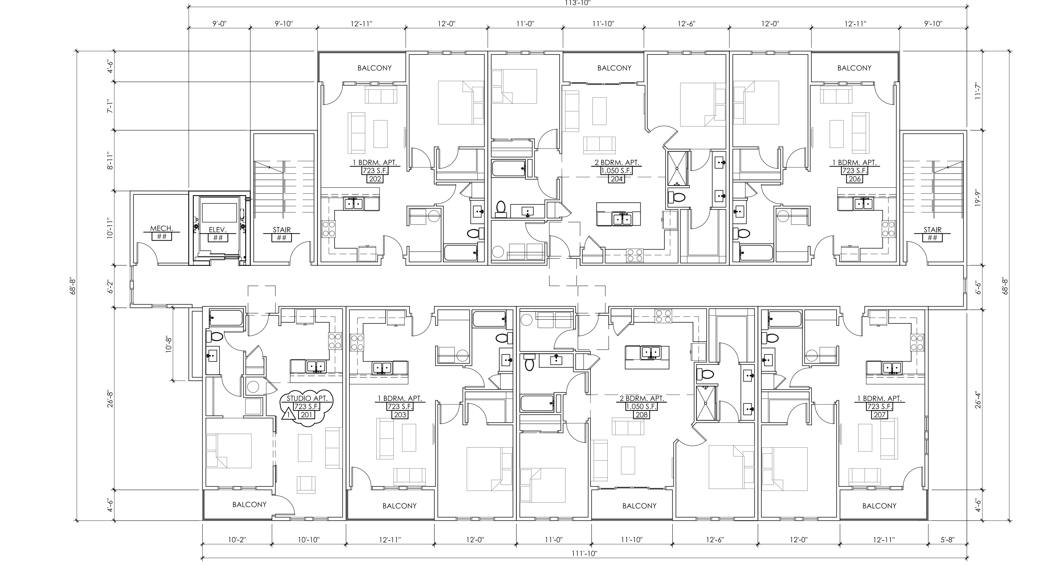
BUILDING 'A' SECOND FLOOR PLAN SCALE: 1/8"=1'-0" * ALL INTERIOR PARTITIONS WILL BE 10'-0" HIGH U.N.O.
