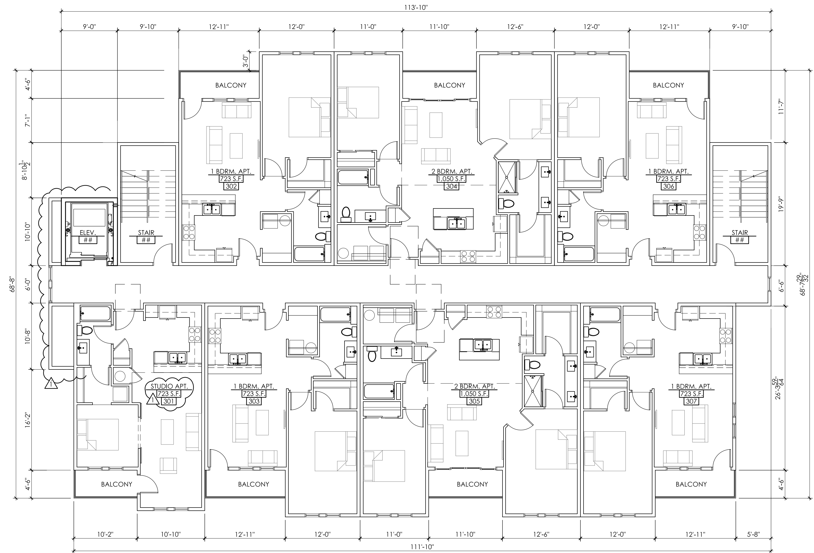
1 BUILDING 'A' & 'B' THIRD FLOOR PLAN A1.2 SCALE: 1/8"=1'-0" * ALL INTERIOR PARTITIONS WILL BE 10'-0" HIGH U.S.O.
