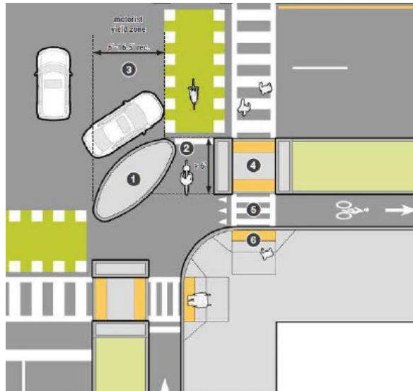
Figure 2 – Protected intersection typical features
