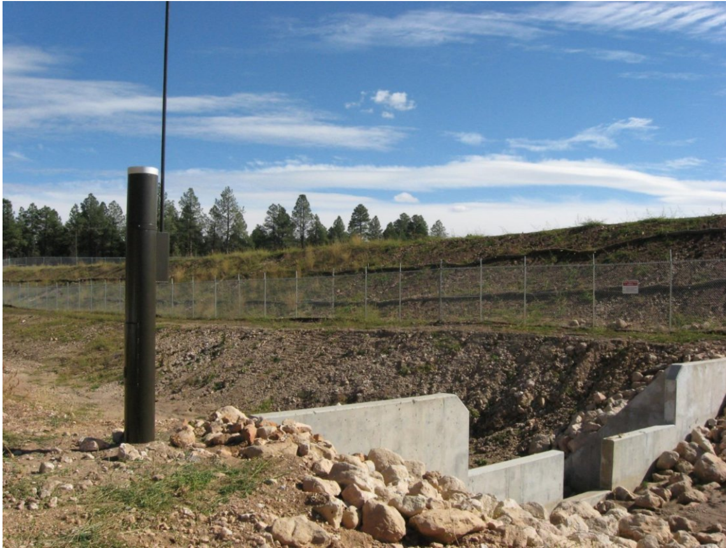
Example photo of a rain and stream gauge installed at a detention basin.
