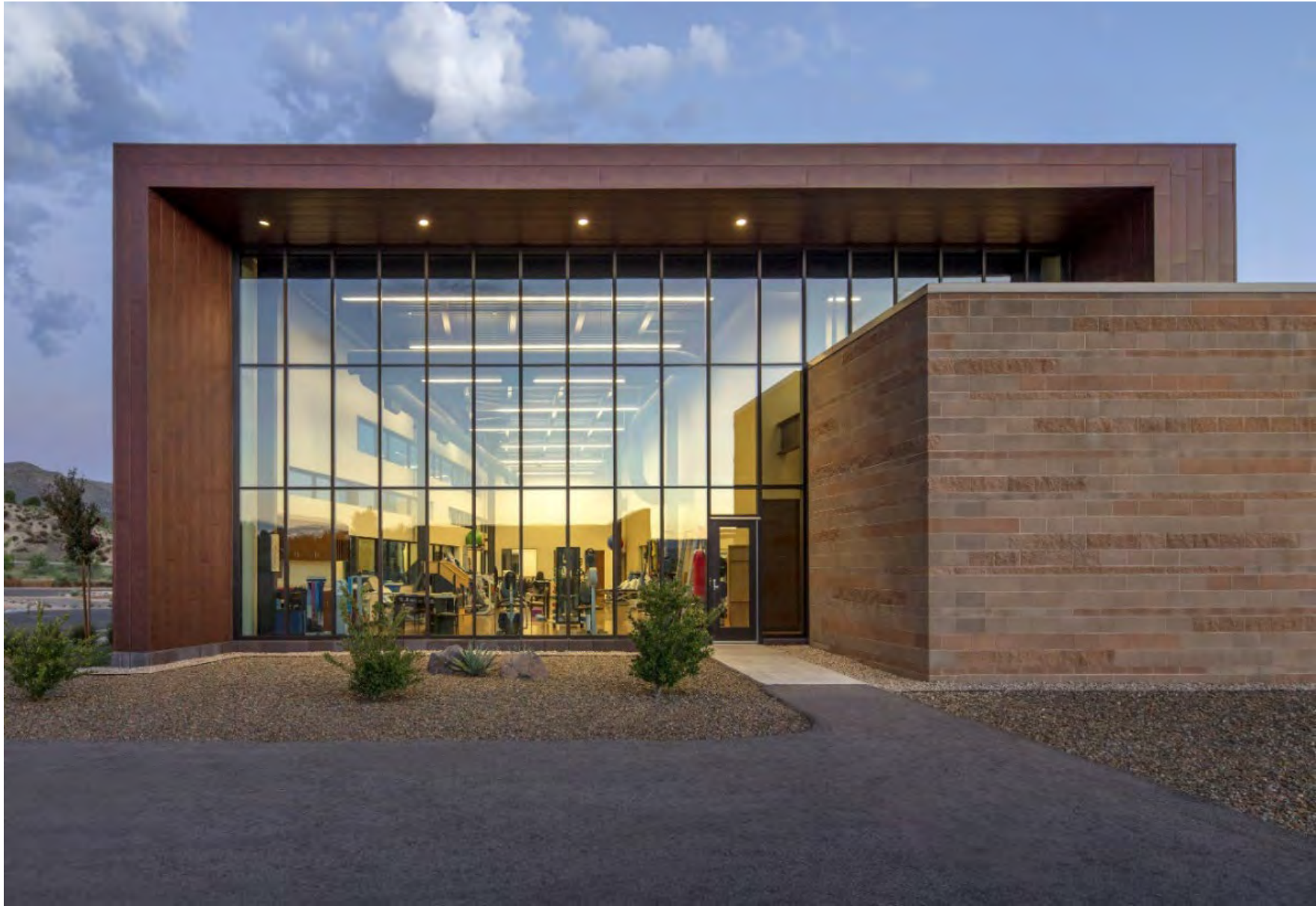
Image 50, Warm colored metal panels, textured masonry, dark window framing, deep horizontal and vertical projections.
