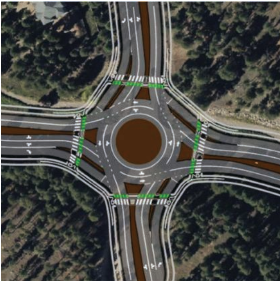
2x2 roundabout with right turn lanes
