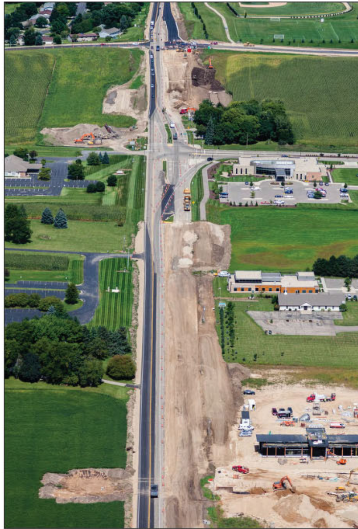
Traditional 4-lane widening with signals
