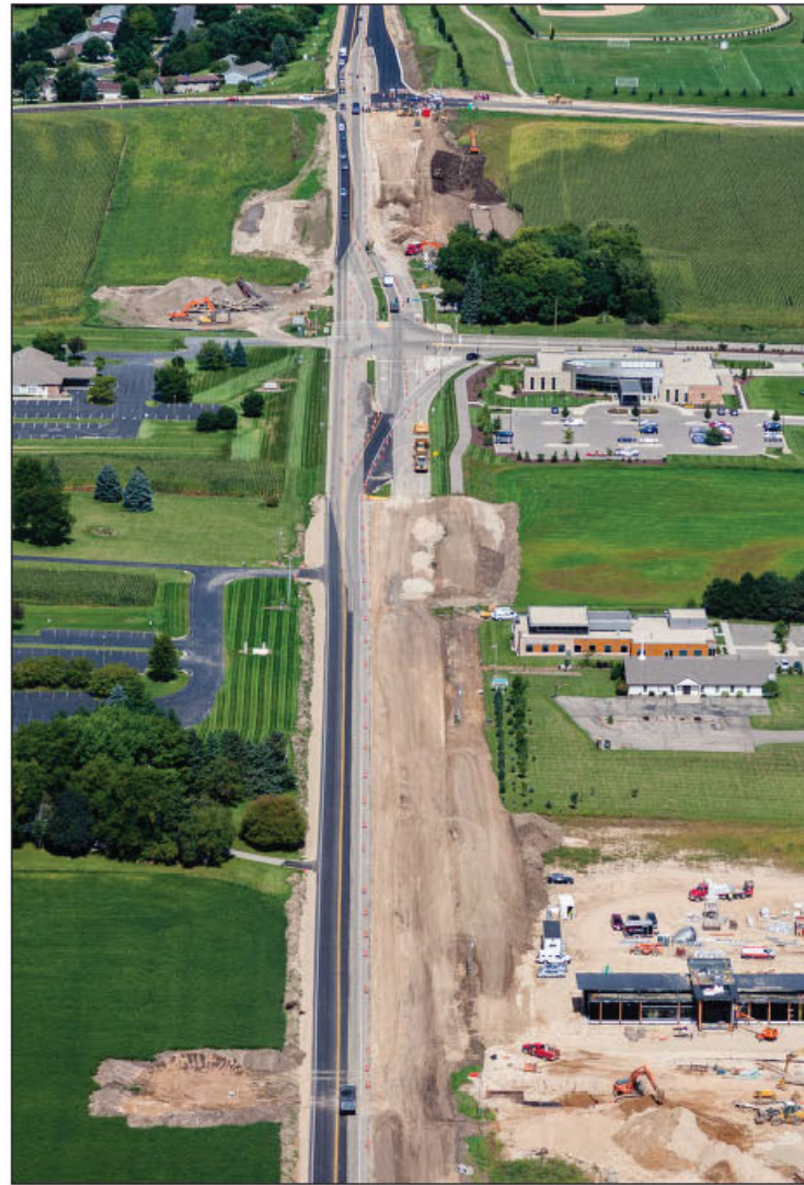
Traditional 4-lane widening with signals
