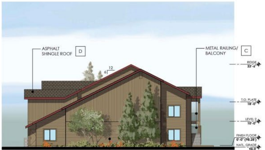
BUILDING TYPE 1 EAST ELEVATION
