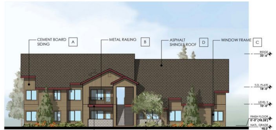
BUILDING TYPE 1 WEST ELEVATION - ISABEL STREET
