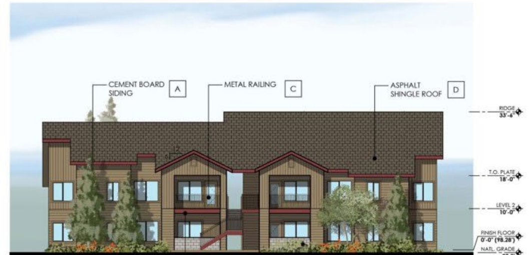
BUILDING TYPE 1 EAST ELEVATION
