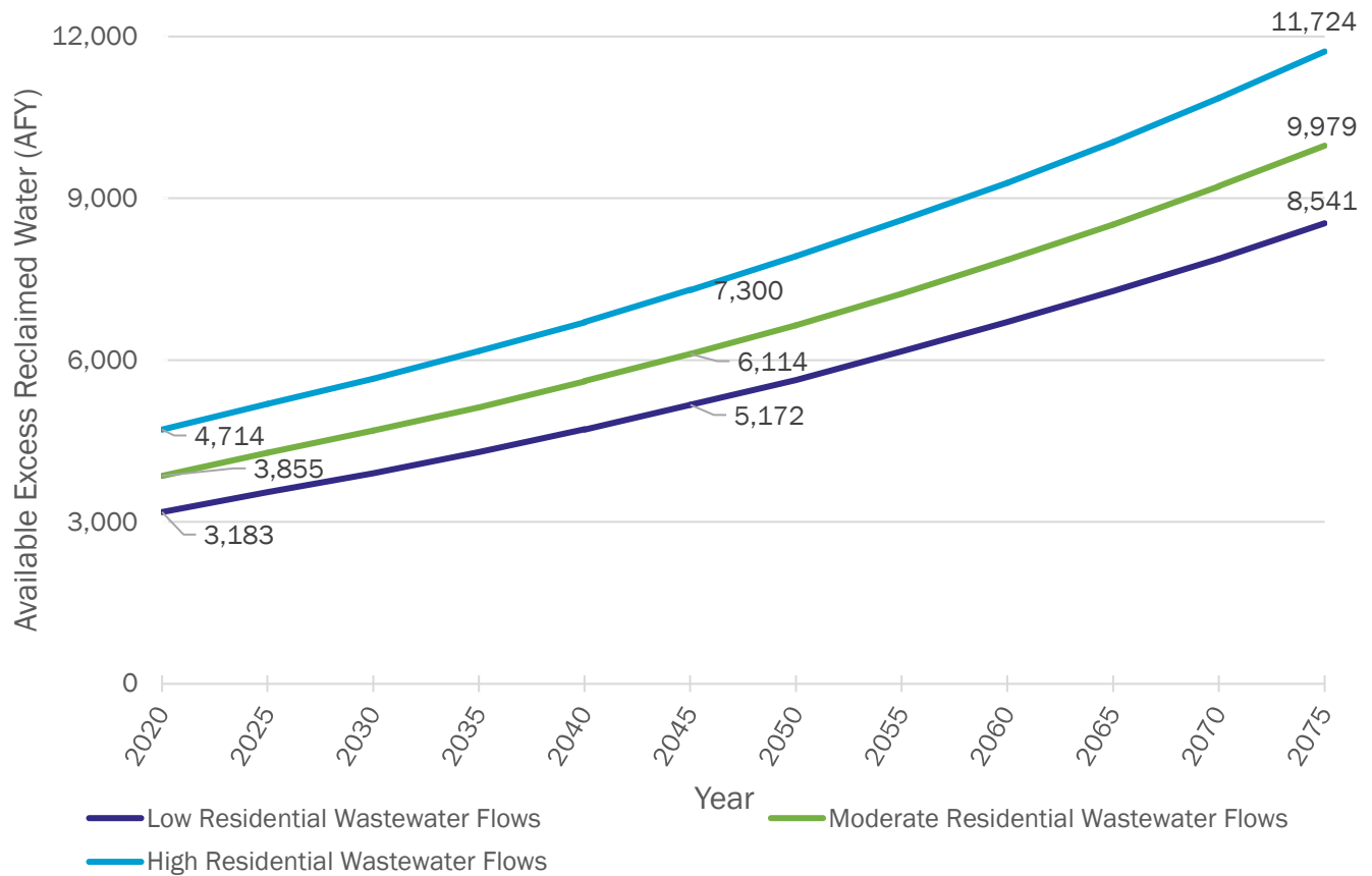
Figure 2-4. Available excess reclaimed water through buildout under low, moderate, and high residential wastewater flow scenarios
