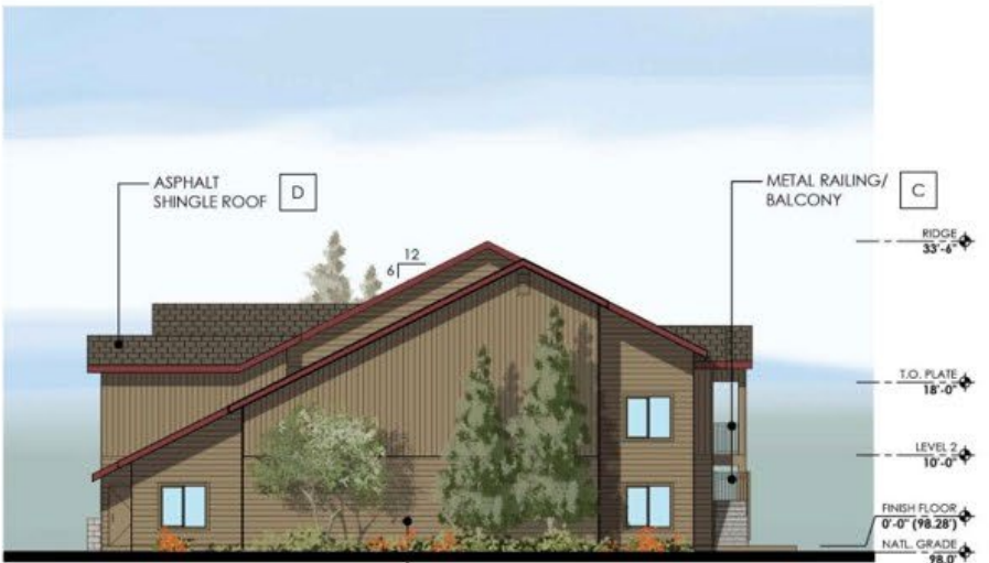
BUILDING TYPE 1 EAST ELEVATION
