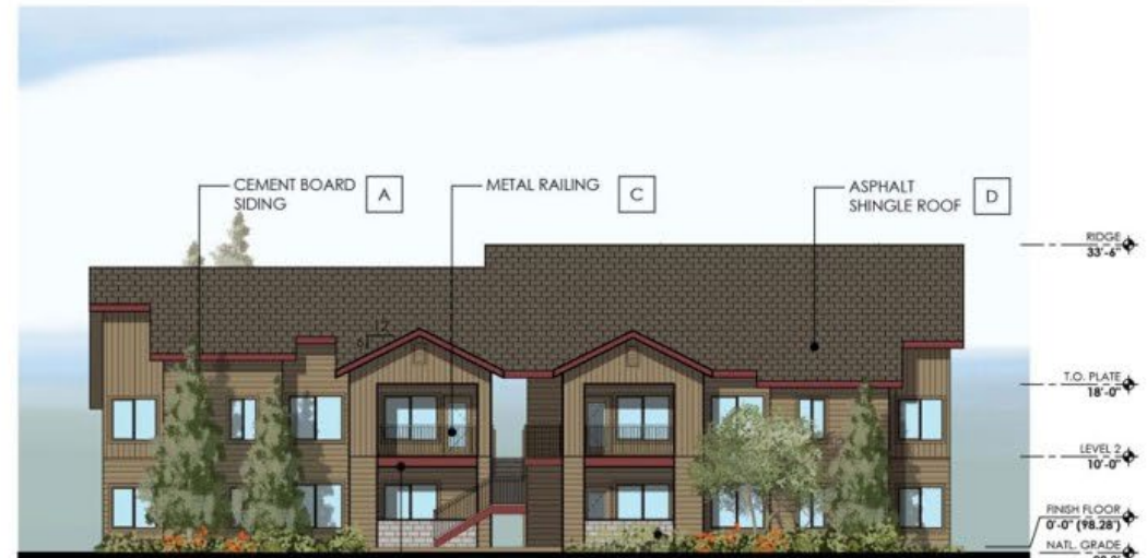
BUILDING TYPE 1 EAST ELEVATION
