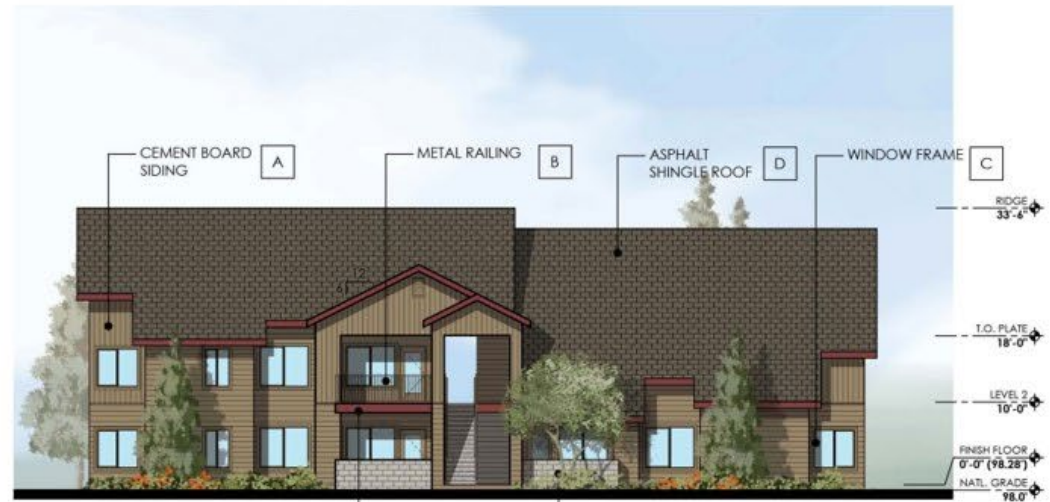
BUILDING TYPE 1 WEST ELEVATION - ISABEL STREET
