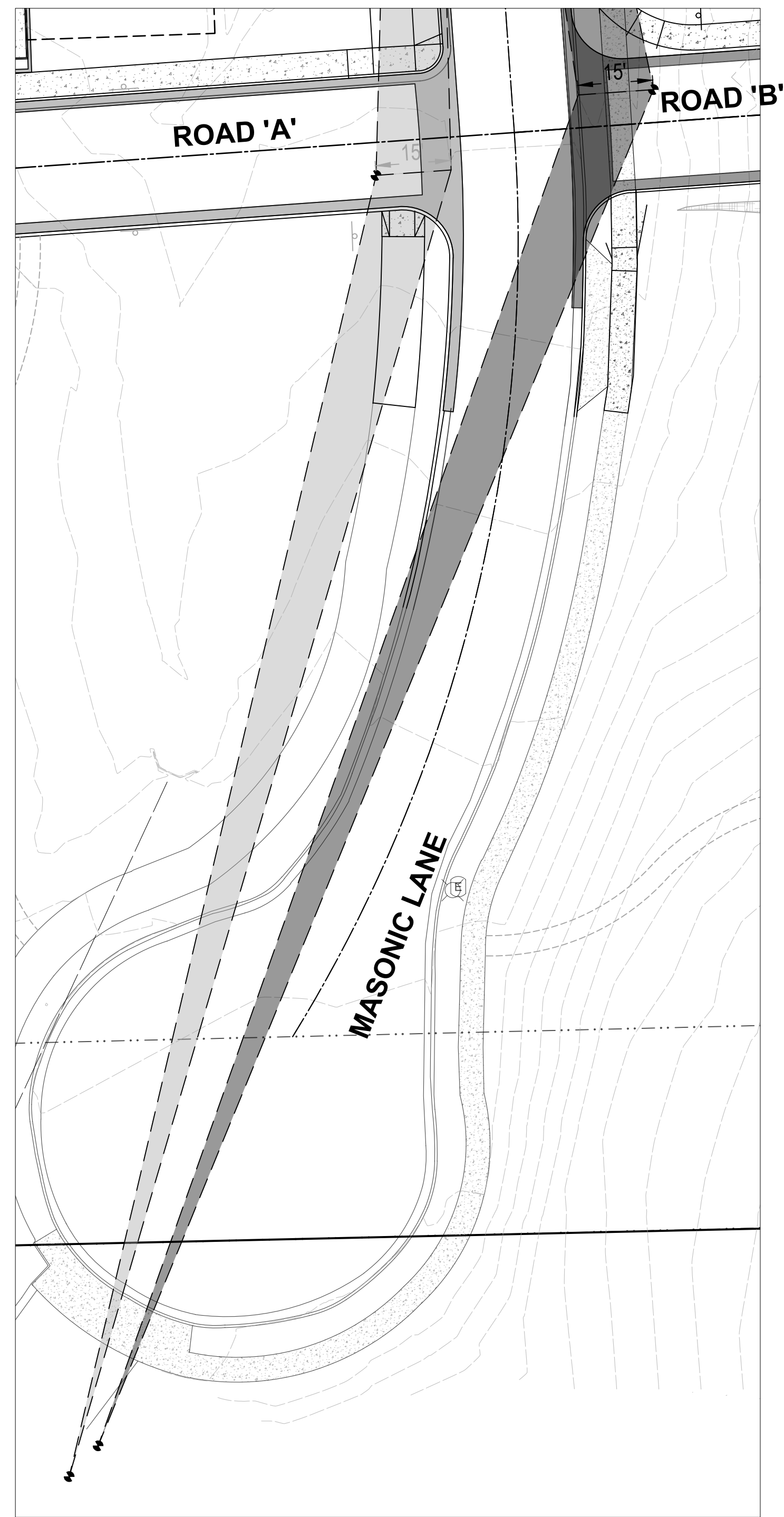
B1 CLEAR VIEW ZONE ROAD 'A' & MASONIC LANE (RIGHT) ROAD 'S' & MASONIC LANE (LEFT) SCALE: 1" = 30'
