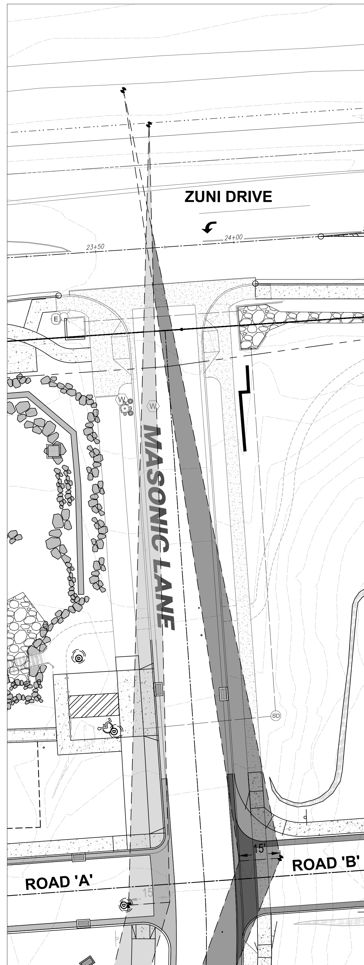
B1 CLEAR VIEW ZONE ROAD 'A' & MASONIC LANE (LEFT) ROAD 'S' & MASONIC LANE (RIGHT) SCALE: 1" = 30'
