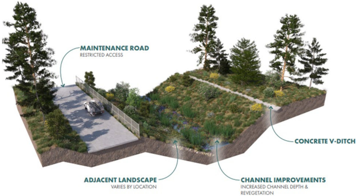
South phase with channel and maintenance road
