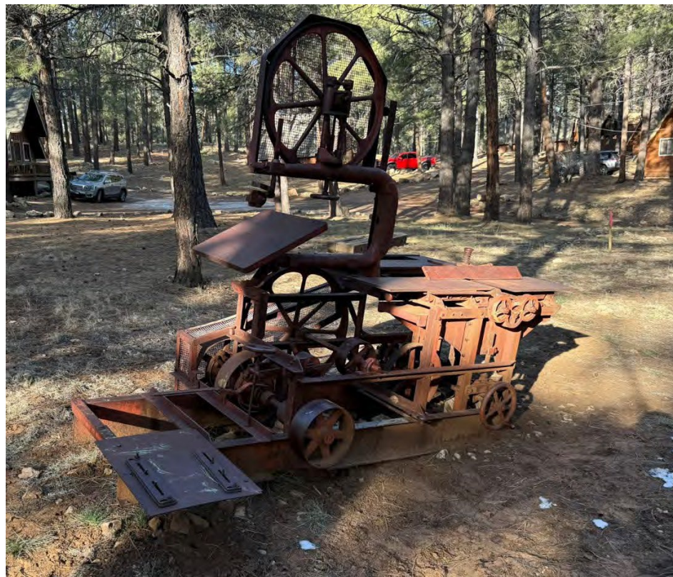
Figure 13 Table saw, jig saw, planer combination (IO9), view west.
