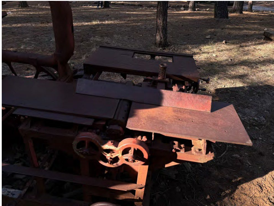
Figure 31 Table saw, jig saw, planer combination (IO9), view west.
