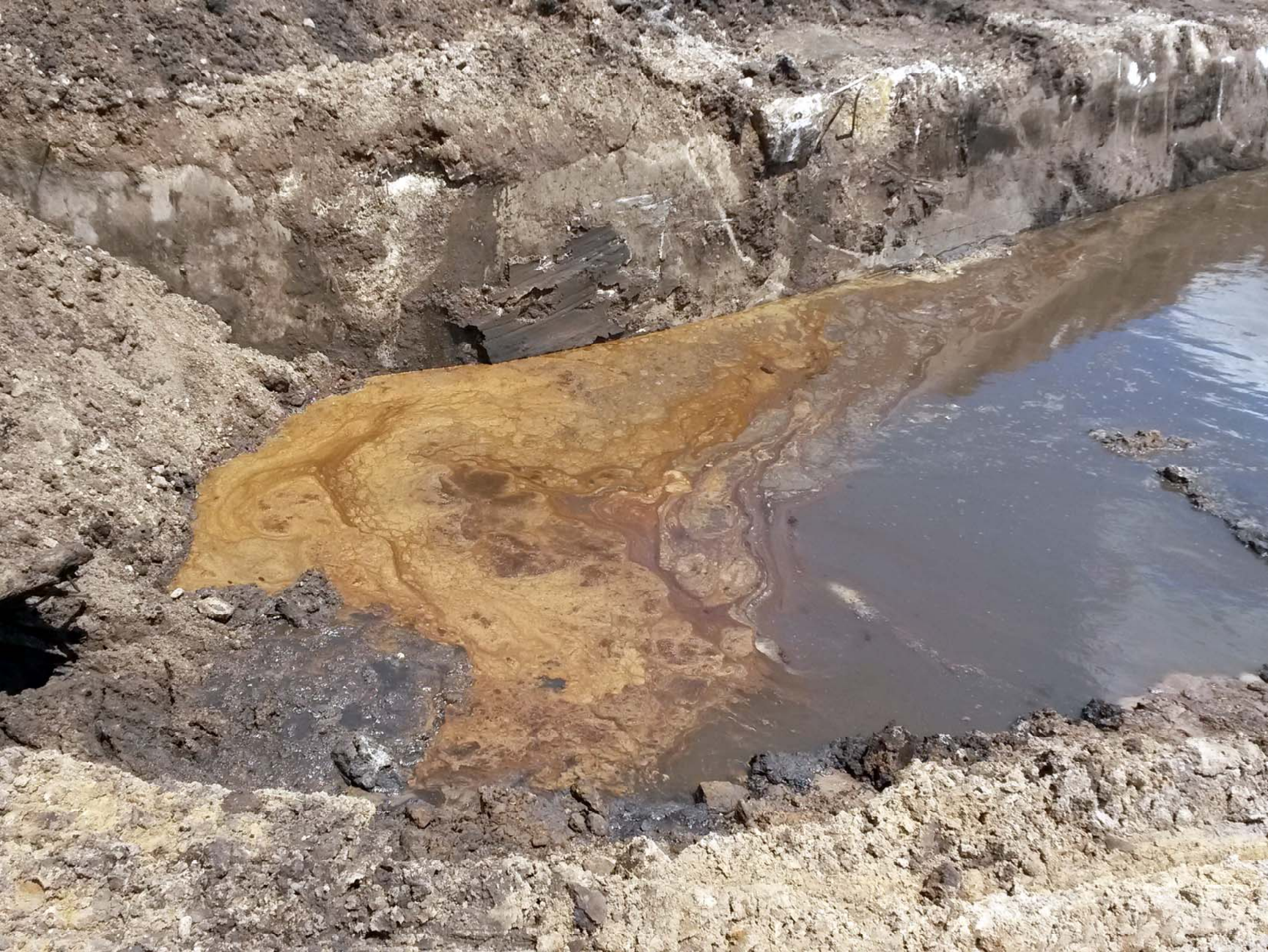
King Plant Property - Petroleum product mixed with ground water - April 10, 2014
