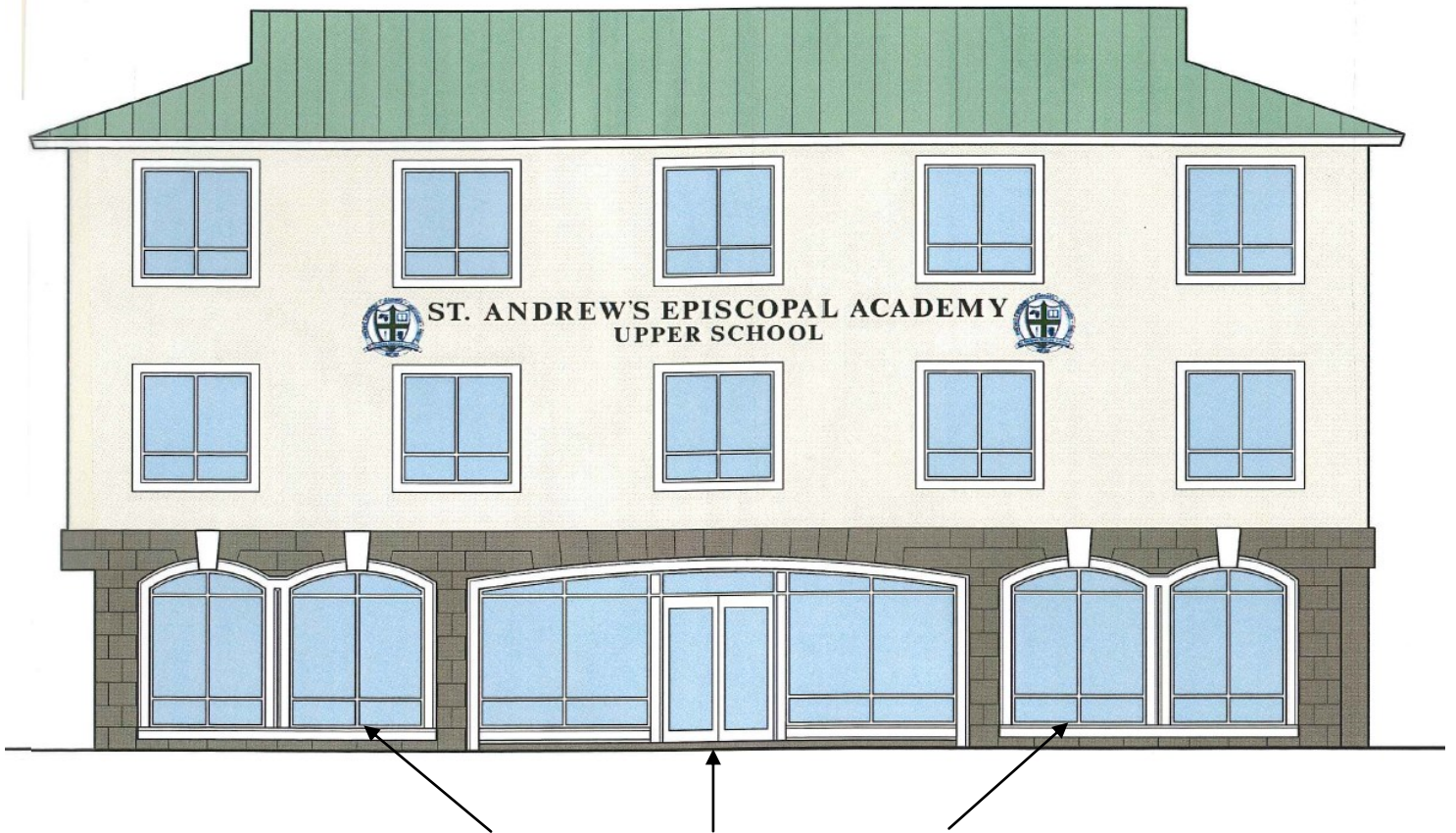
Addition of Store front Doors and Windows consistent with the established design
