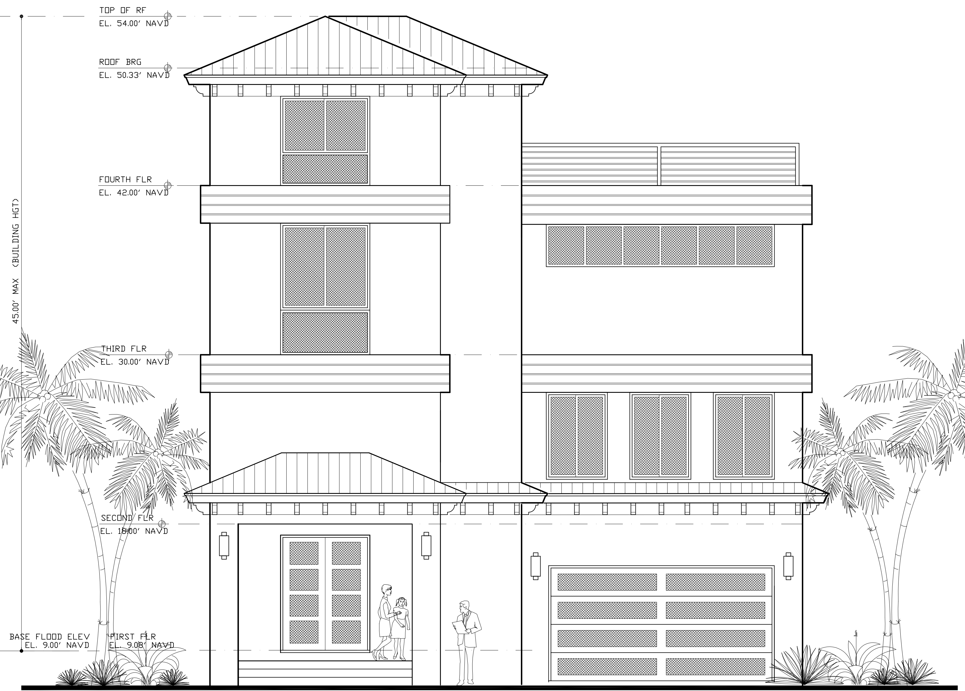
WEST FRONT ELEVATION SCALE: 1/4" = 1'-0"
