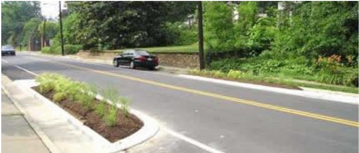
Exhibit 3.8 - Typical Mid-Block Choker Application:
