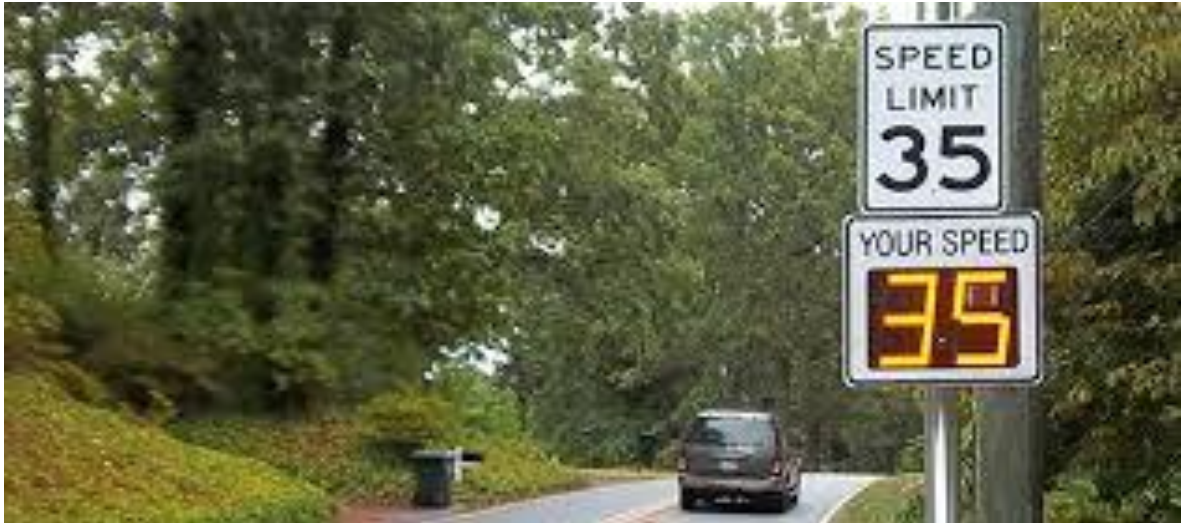
Exhibit 4.3 – Radar Speed Feedback Sign:
