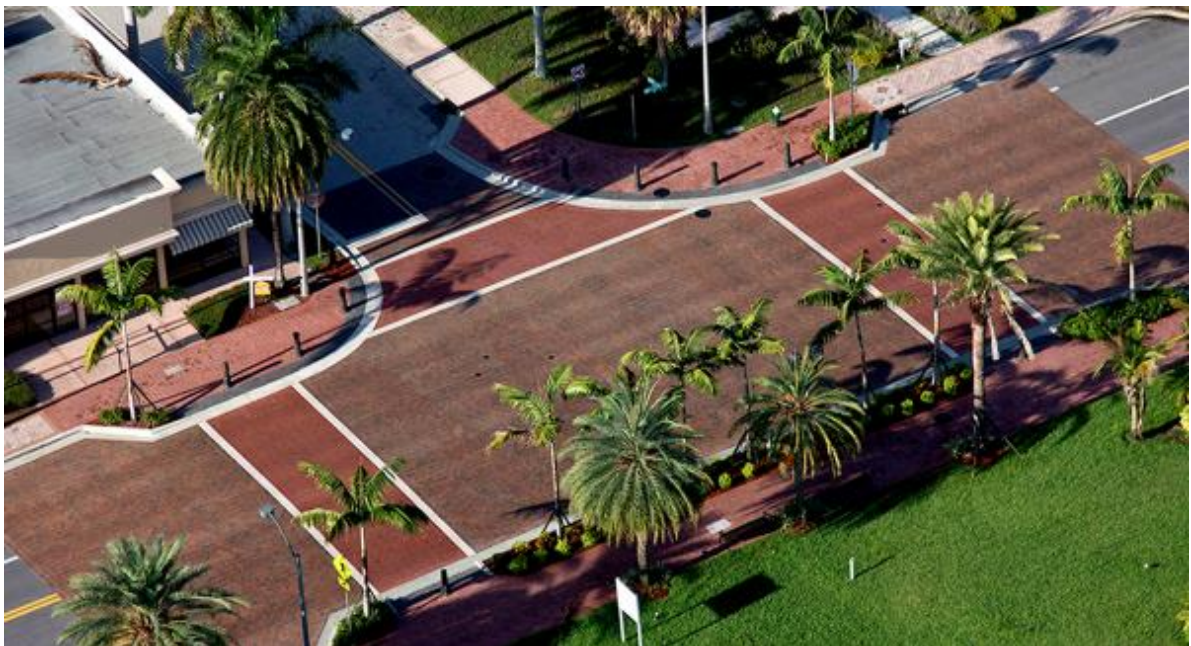
Exhibit 3.3 - Typical Speed Hump Application:
