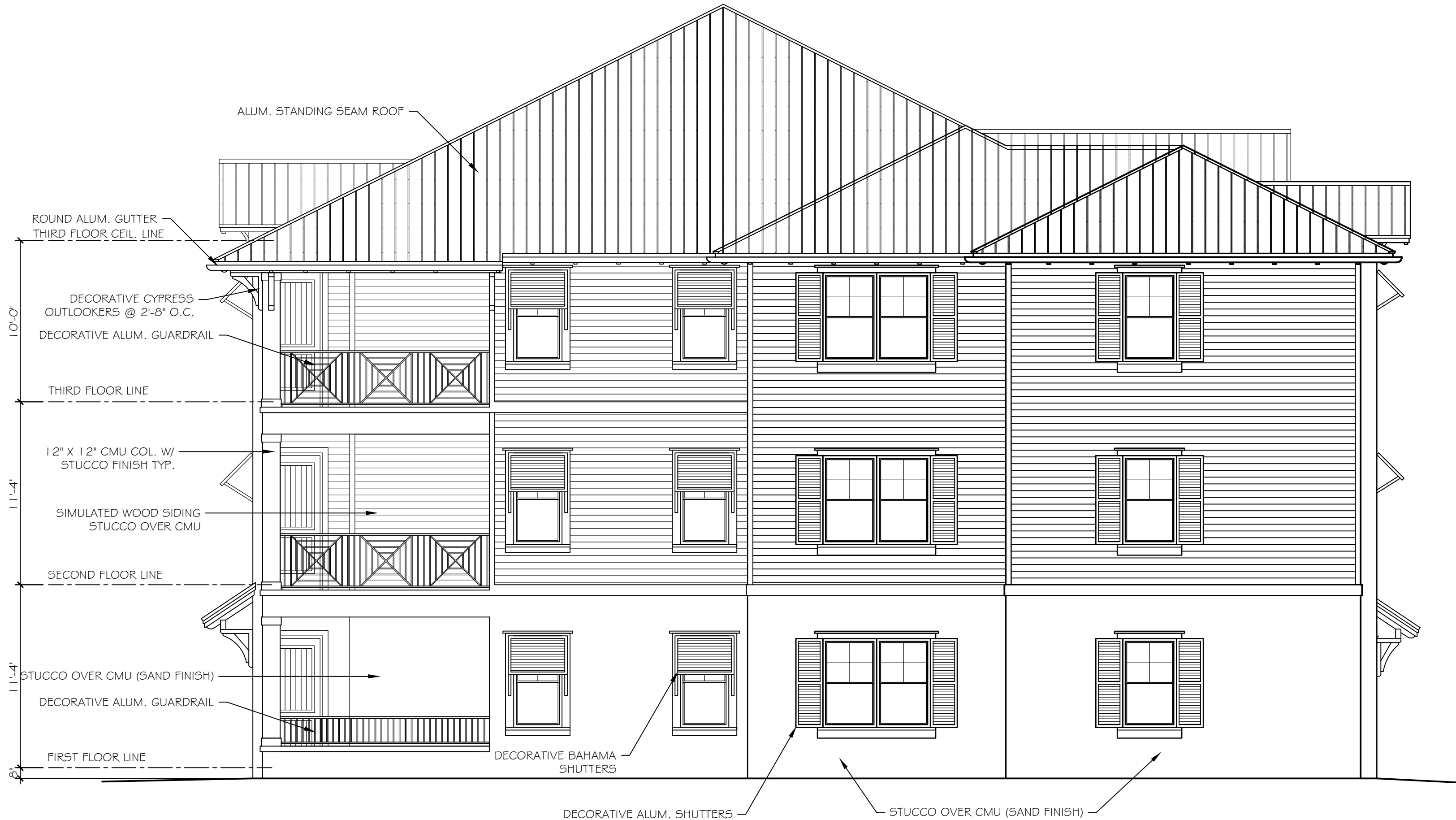
1 LEFT (NORTH) ELEVATION 3/16" = 1'-0" NOTE: REFER TO RENDERING FOR COLORS
