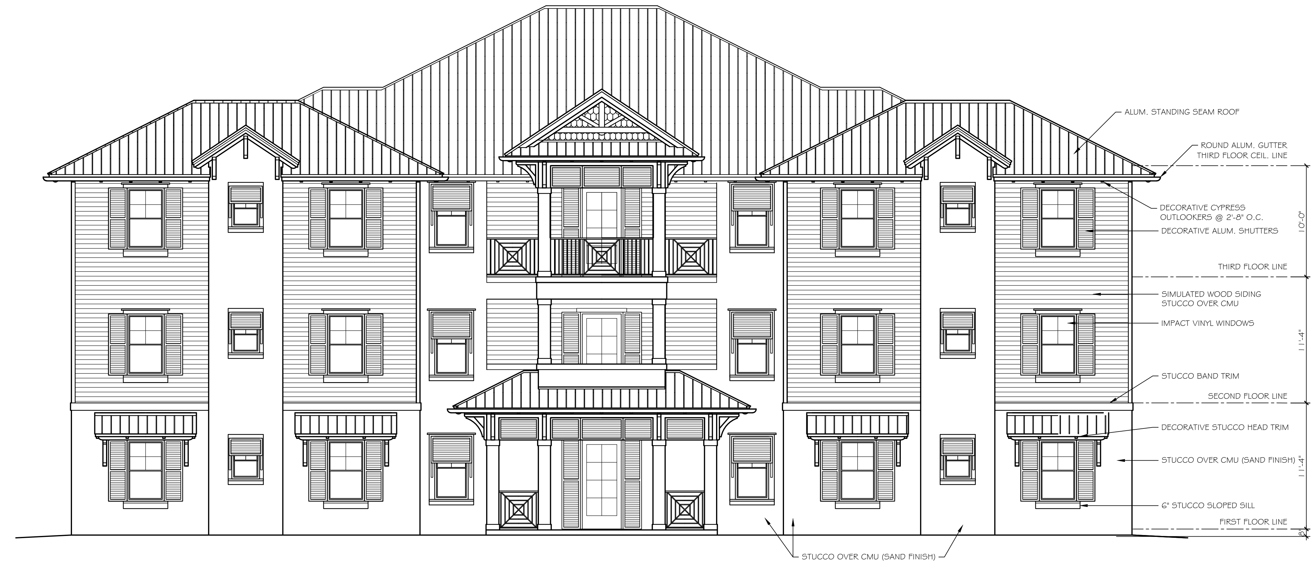
1 FRONT (WEST) ELEVATION 3/16" = 1'-0" NOTE: REFER TO RENDERING FOR COLORS
