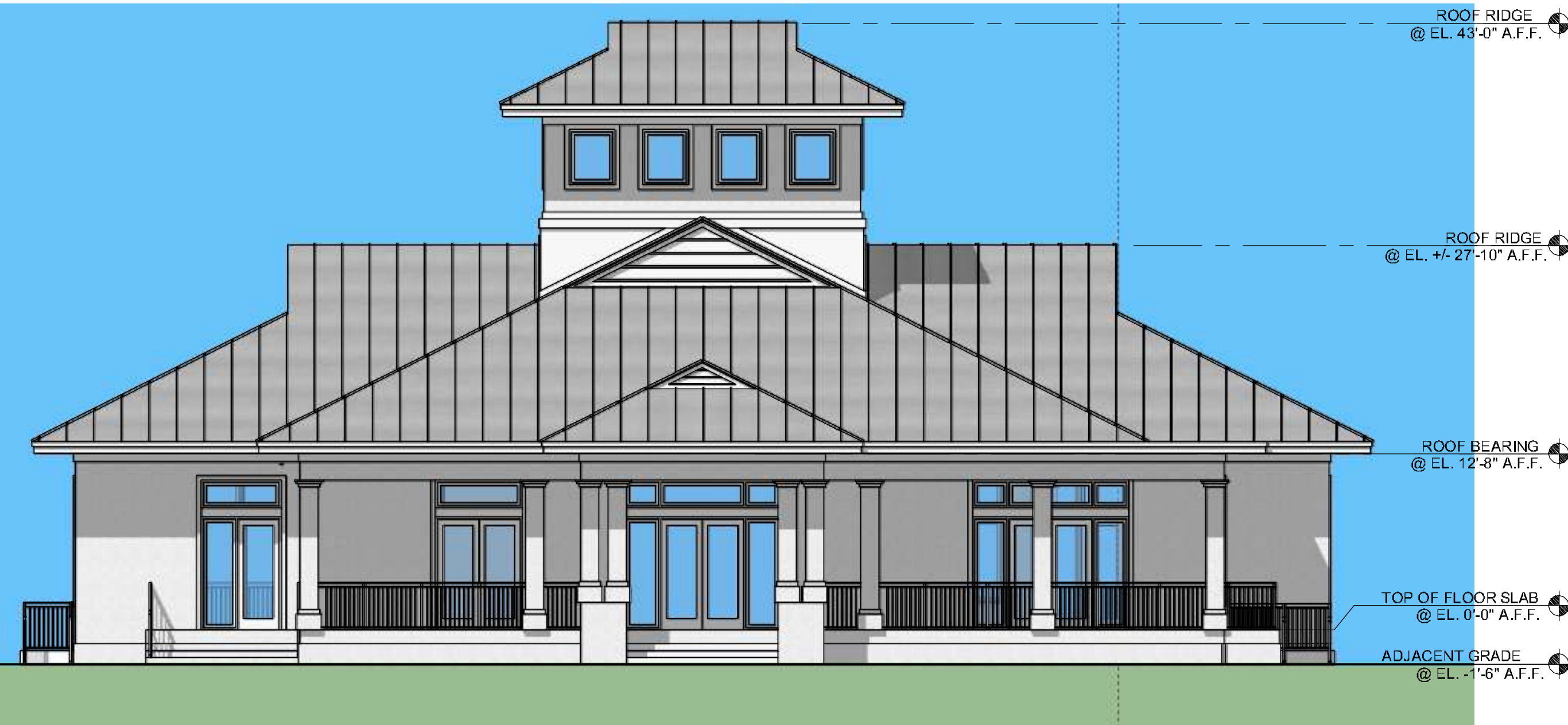
EAST BUILDING ELEVATION SCALE: 1/8" = 1'-0" B A-2.01
