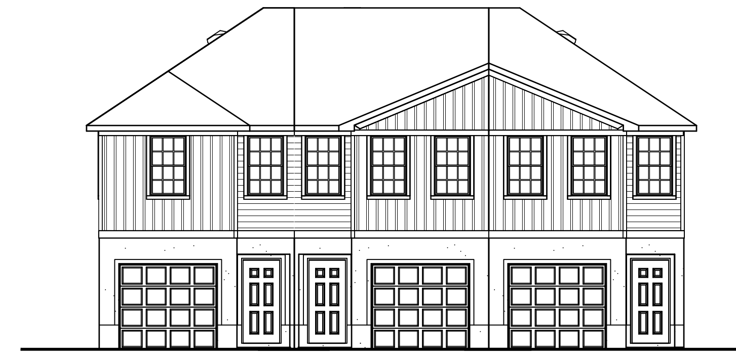
UNIT C ELEVATION "A" (PER PLAN) UNIT B ELEVATION "B" (REVERSE) UNIT A ELEVATION "B" (PER PLAN) 3 B-2 3 - UNIT BUILDING SCALE: 1/8" = 1'-0" FL603
