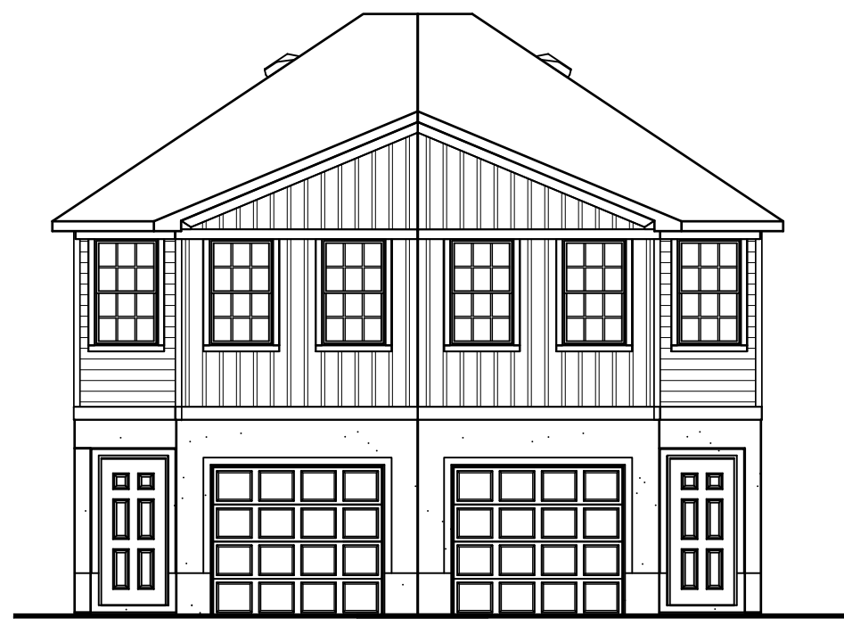
UNIT B ELEVATION "B" (REVERSE) UNIT A ELEVATION "B" (PER PLAN) 2 B-2 2 - UNIT BUILDING SCALE: 1/8" = 1'-0" FL62B
