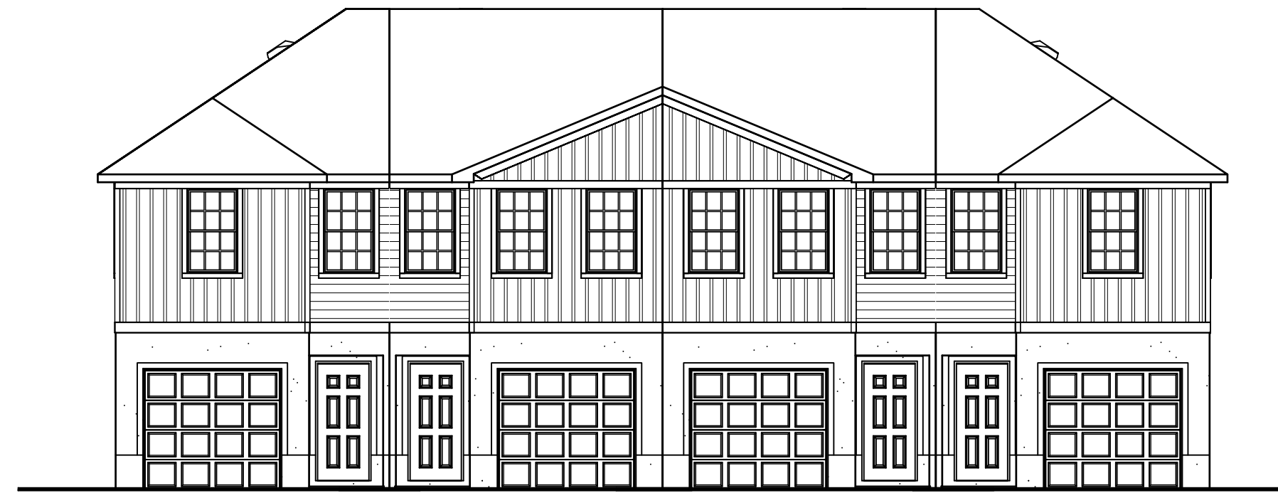
UNIT D ELEVATION "A" (PER PLAN) UNIT C ELEVATION "B" (REVERSE) UNIT B ELEVATION "B" (PER PLAN) UNIT A ELEVATION "A" (REVERSE) 4 B-2 4 - UNIT BUILDING SCALE: 1/8" = 1'-0" FL604
