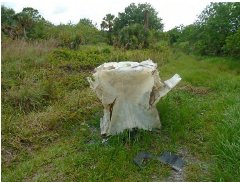
7. West View: 250-Gallon HDPE Chemical Storage Tote on the Subject Property Note: The HDPE Tote Appeared Empty and Damaged with Vegetation Growing inside
