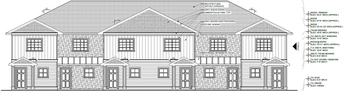
1 TH2C - FRONT ELEVATION TH2C Scale: 1/4" = 1'-0"
